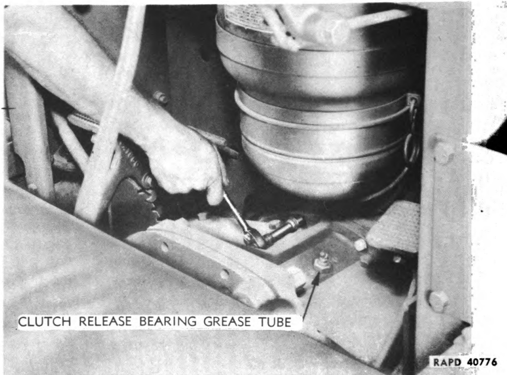
Figure 44—Removing Cap Screw Holding Engine to Spacer
