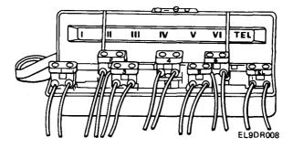
1. Connect the incoming lines to the adapters with the designation strip facing the operator.
