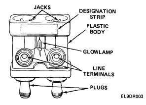
CONNECTOR ADAPTER. A combination jack and plug that fits into the jacks of other adapters, allowing for lineto-line or conference calls. The plugs, which are thumbscrews, secure telephone lines at the line terminal points through clamping force. A glow lamp seated inside the adapter's clear-plastic body will light when an incoming call is received. A designation strip painted on the body of the adapter allows the operator to designate terminal lines in writing.
