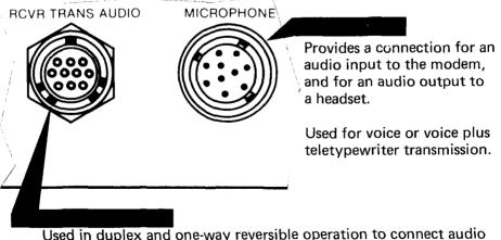
Used in duplex and one-way reversible operation to connect audio output circuit from modem to exciter section of receiver-transmitter.
