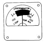
• Tune the receiver and modem BFO (850-Hz mode only) until the meter registers in the DISCRIMINATOR scale during the entire message. (Tune so that the indicator needle swings the maximum range within the discriminator section of the meter. )
