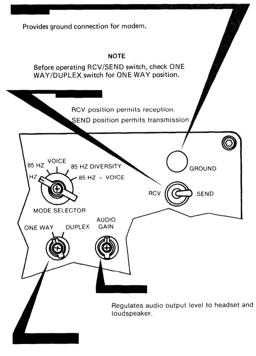
ONE WAY position permits either reception or transmission. DUPLEX position permits reception and transmission at the same time.
