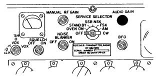
• Check meter to see that correct current flow (20 or 60 mA) is in dc loop no. 2.
