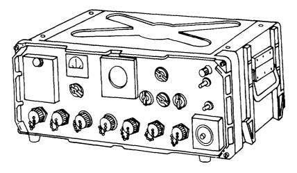
Four feet are on the bottom of the modem case so it may be firmly seated in a modified mounting MT-3140/GRC-106 (used with, but not part of, the modem).
