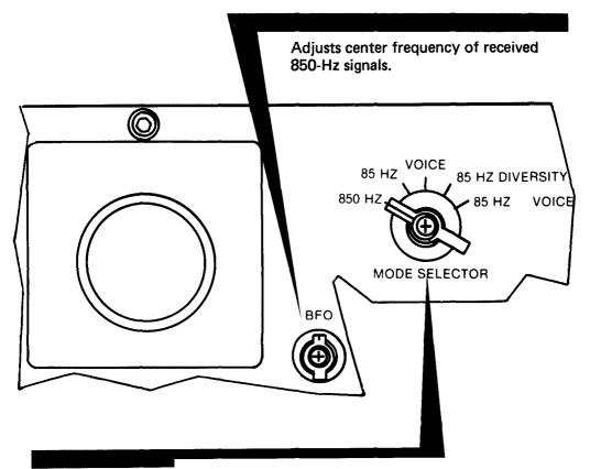
The position of this switch selects the mode of operation.
