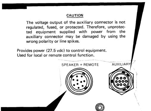
Provides connection for an audio input to the modem and for an audio output to loudspeaker. May be used with other equipment for remote operation.
