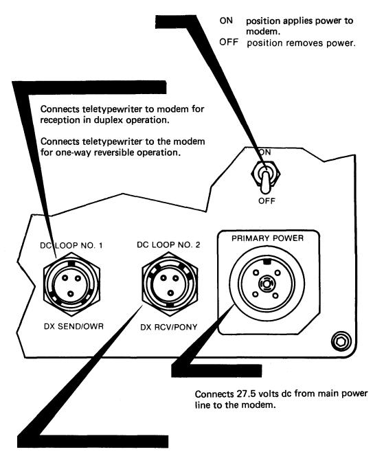
Connects teletypewriter to modem for reception in duplex operation.
