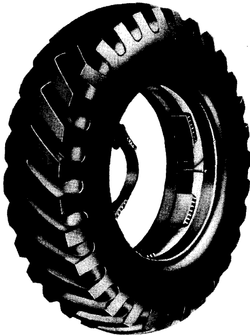
Figure 118 — Removing Bead Lock
