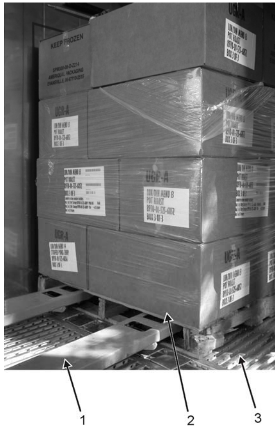
Figure 27. Pallets 9 and 10 Lift and Place.
