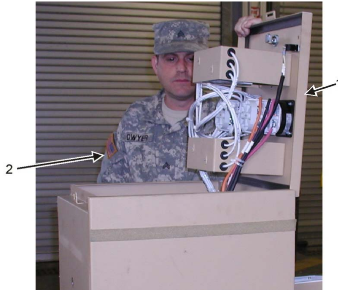
Figure 16. Power Box Door.
