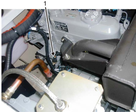
Figure 9. Oil Pressure Safety Switch.
