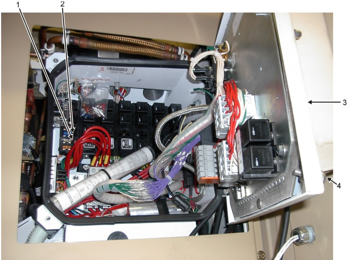
Figure 5. MPC Box Fuses.
