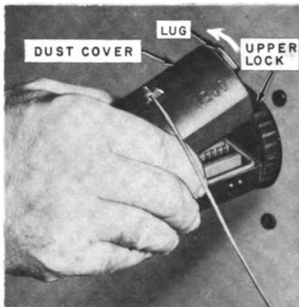
C. REMOVAL OF DUST COVER.
