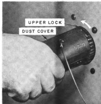
B. UNLOCKING UPPER LOCK.
