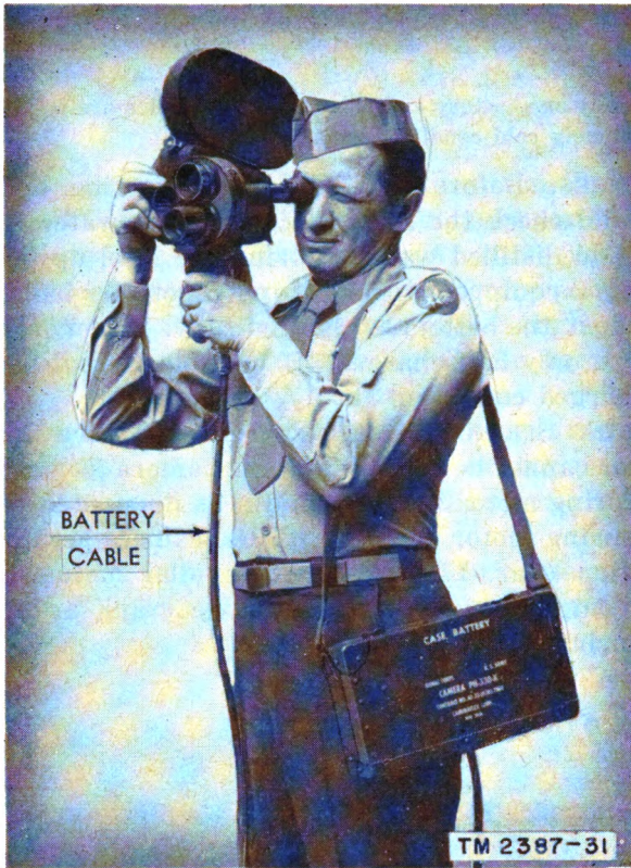
Figure 13. Correct position for hand-held camera.
