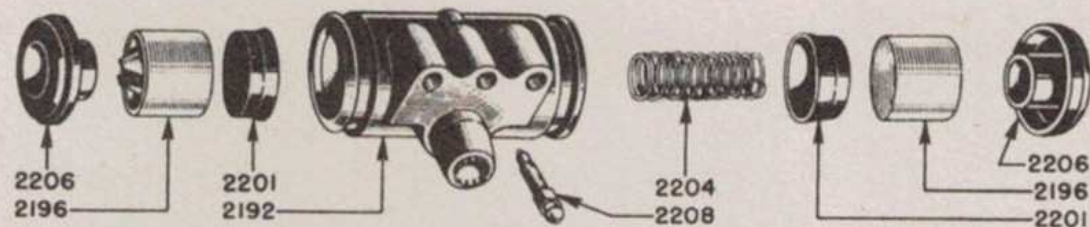
Exploded View of Wheel Cylinder-- Fig. 18 TO REMOVE THE WHEEL CYLINDER
