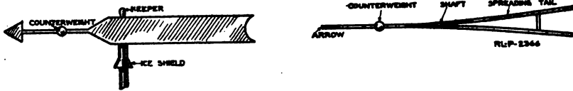
Fig. 24.—Side elevation and plan of wind vane
