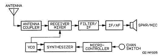
Figure 4-1. Receiver Operation, Simplified Block Diagram
