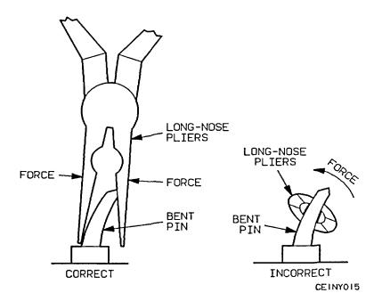
Figure 5-4. Pin Straightening Technique
