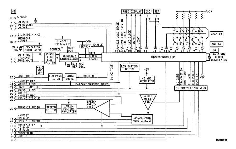
Figure 4-4. Synth/AF Module Block Diagram
