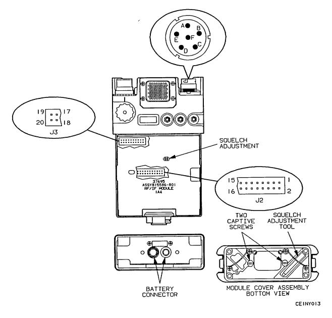
Figure 5-3. Radio Set Component Locations Diagram (Sheet 1 of 2)
