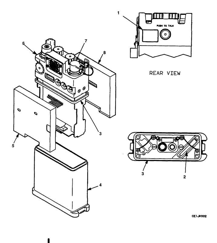
Figure C-2. Receiver-Transmitter RT-1547/PRC-126
