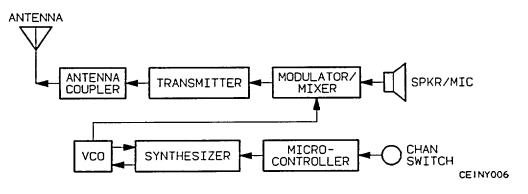
Figure 4-2. Transmitter Operation, Simplified Block Diagram
