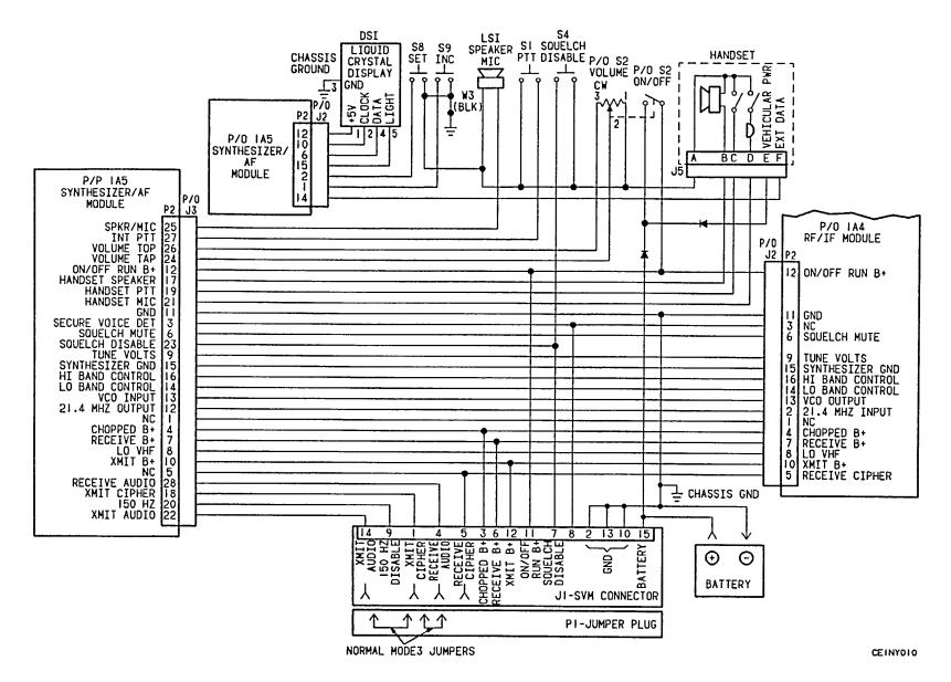
Figure 4-5. Radio Set Interconnect Diagram (Sheet 2 of 2)
