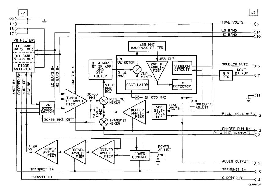
Figure 4-3. RF/IF Module Block Diagram
