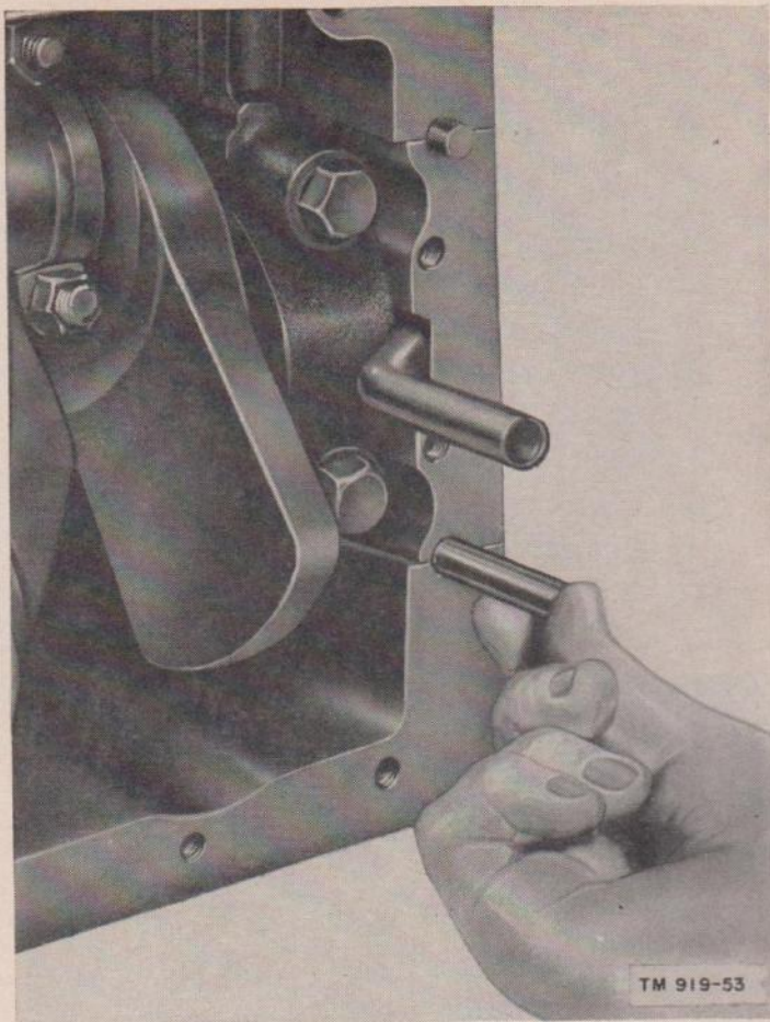
Figure 54. Installing rear main-bearing cap packing.
