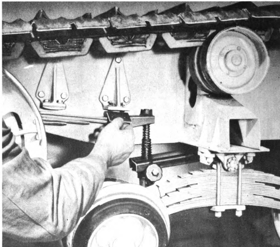
Figure 107—Shimming Spring Stop Bracket to Adjust Track Tension
