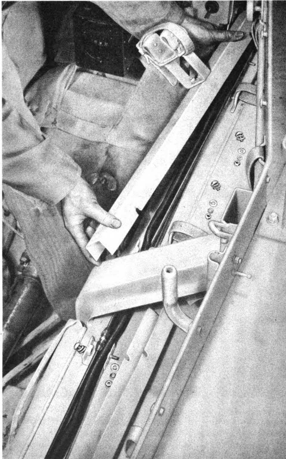
Figure 153—Removing Conduit Covers
