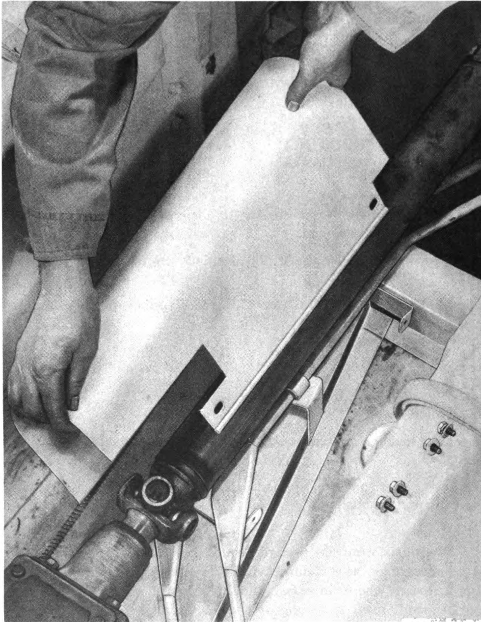
Figure 32—Removing Propeller Shaft Cover
