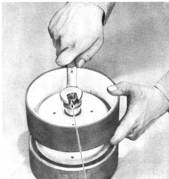
Figure 134—Installing Guide Wheel Bearings
