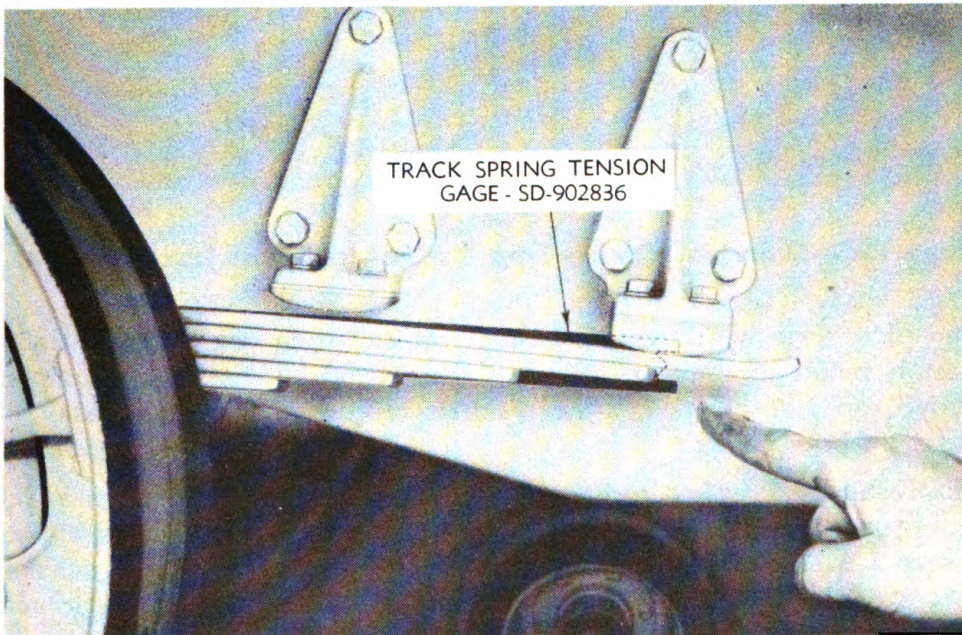
Figure 106—Checking Track Tension
