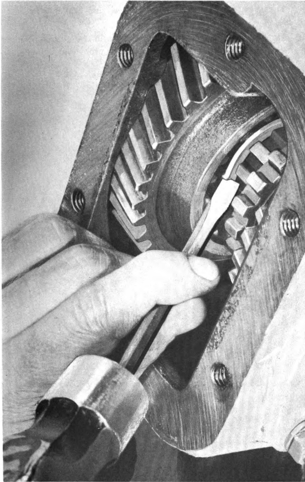
Figure 54—Cutting Pinion Low Speed Gear Snap Ring for Removal
