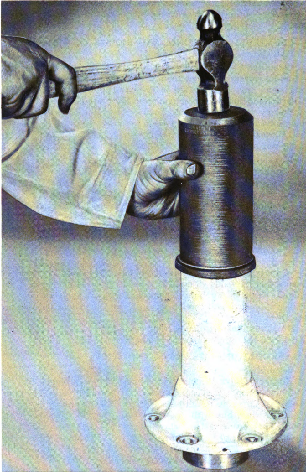
Figure 44—Installing Drive Wheel Carrier Oil Seal
