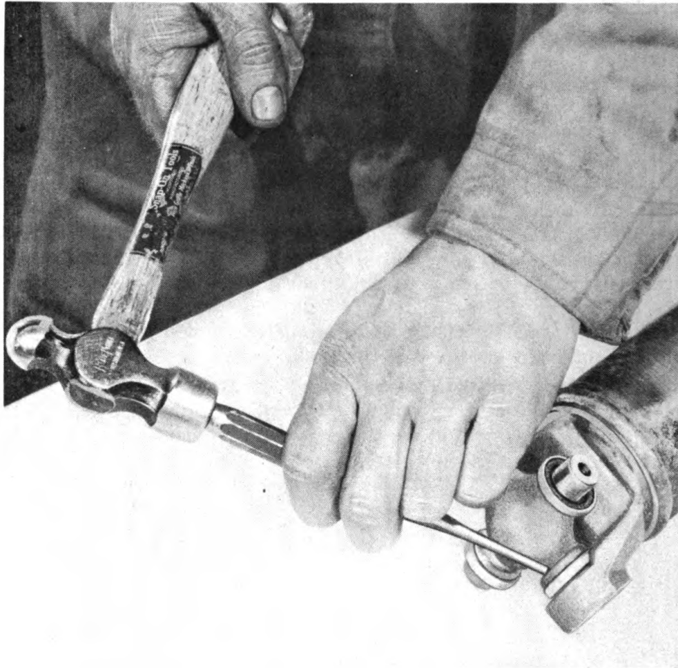
Figure 38—Eliminating Bind at Bearing Seals
