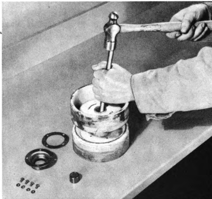
Figure 133—Removing Guide Wheel Bearings
