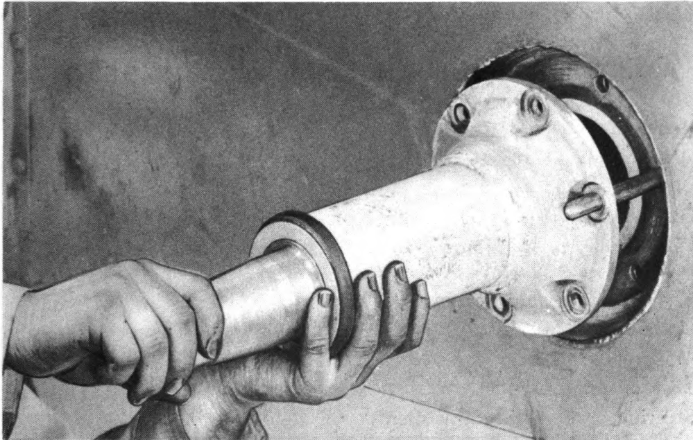
Figure 45—Installing Drive Wheel Carrier
