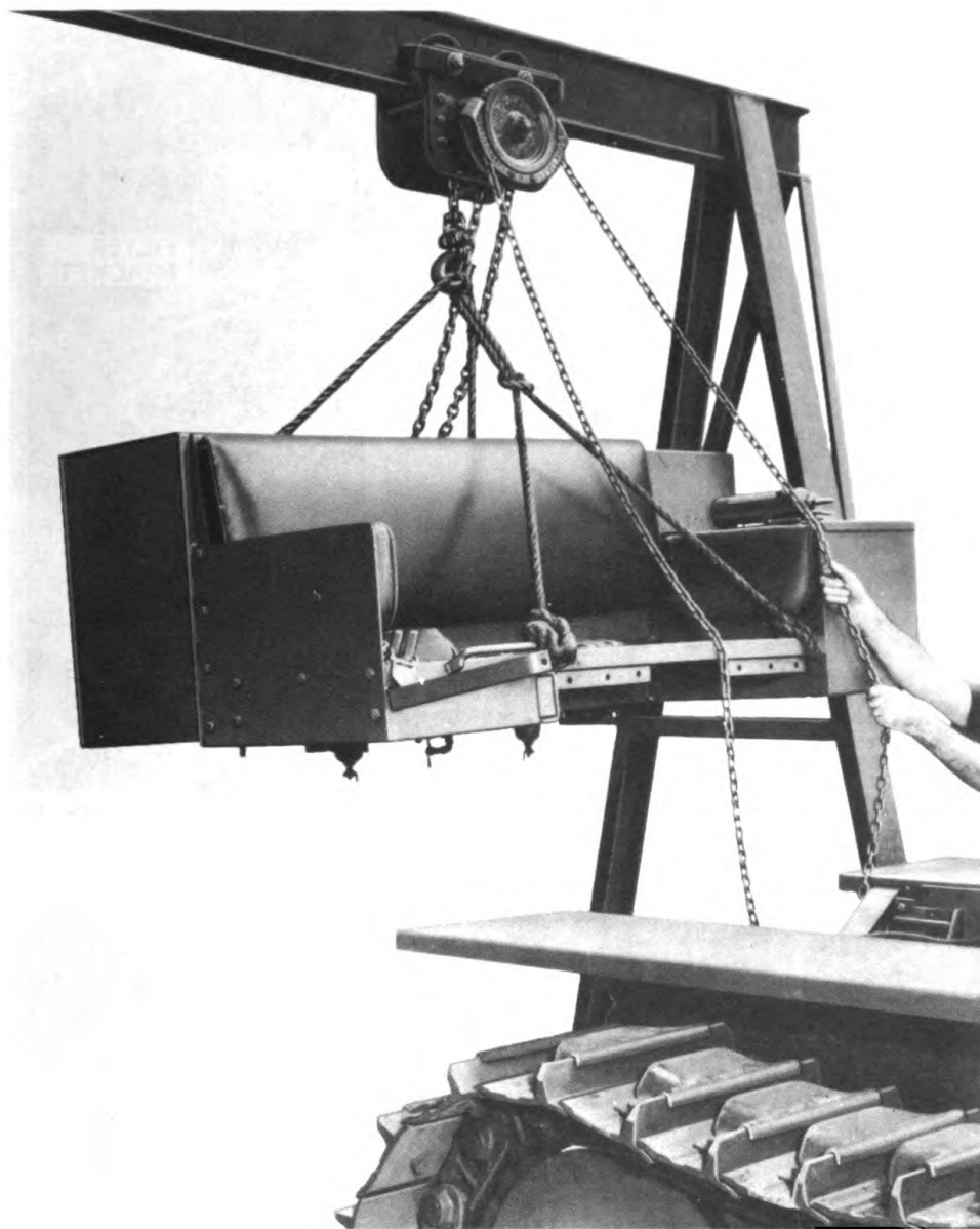
Figure 104 — Lifting off Seat Frame and Fuel Tank Assembly
