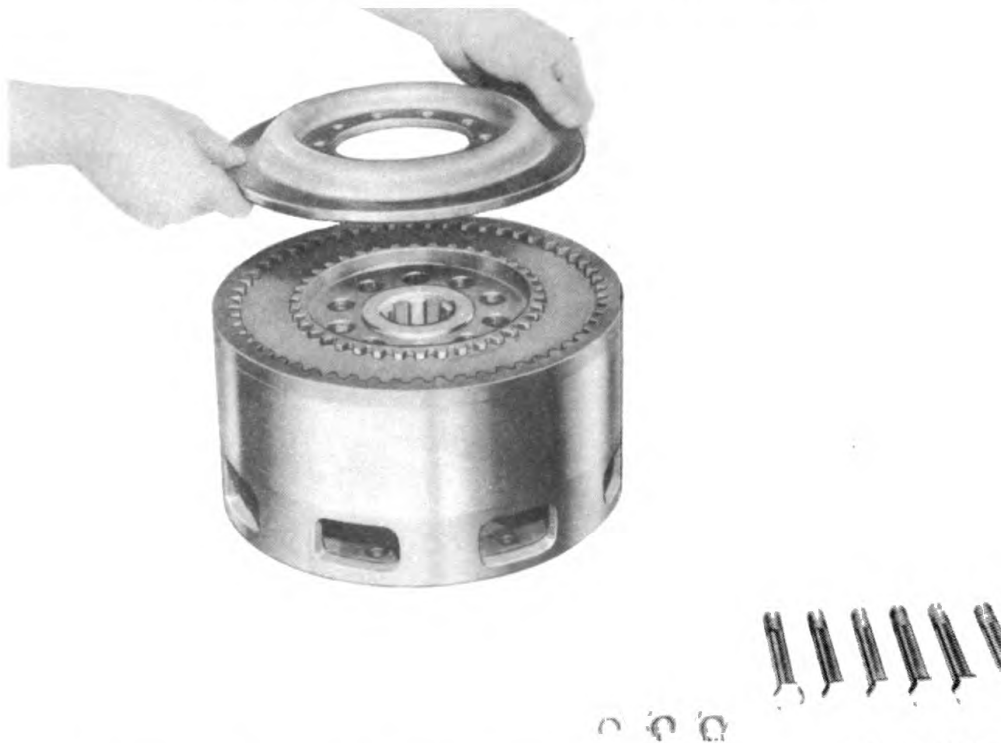
Figure 141 — Installing Pressure Plate on Clutch Disks
