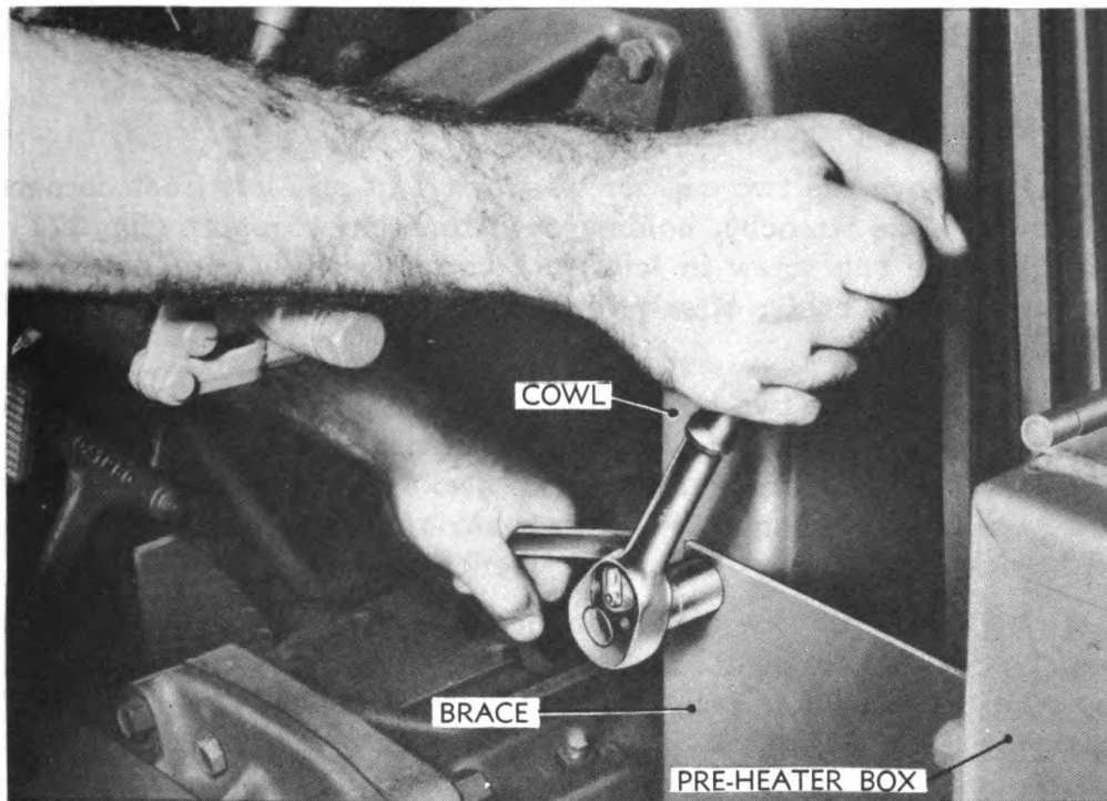
Figure 322 — Removing Bolts from Preheater Box Brace 327
