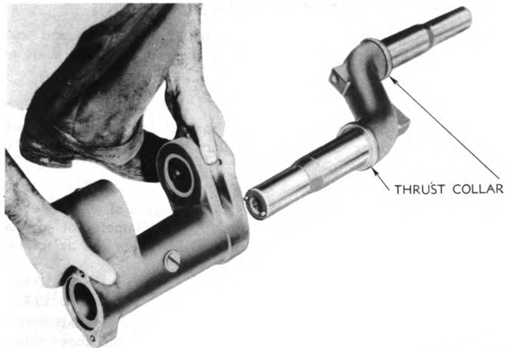
Figure 97 — Link Removed from Crank
