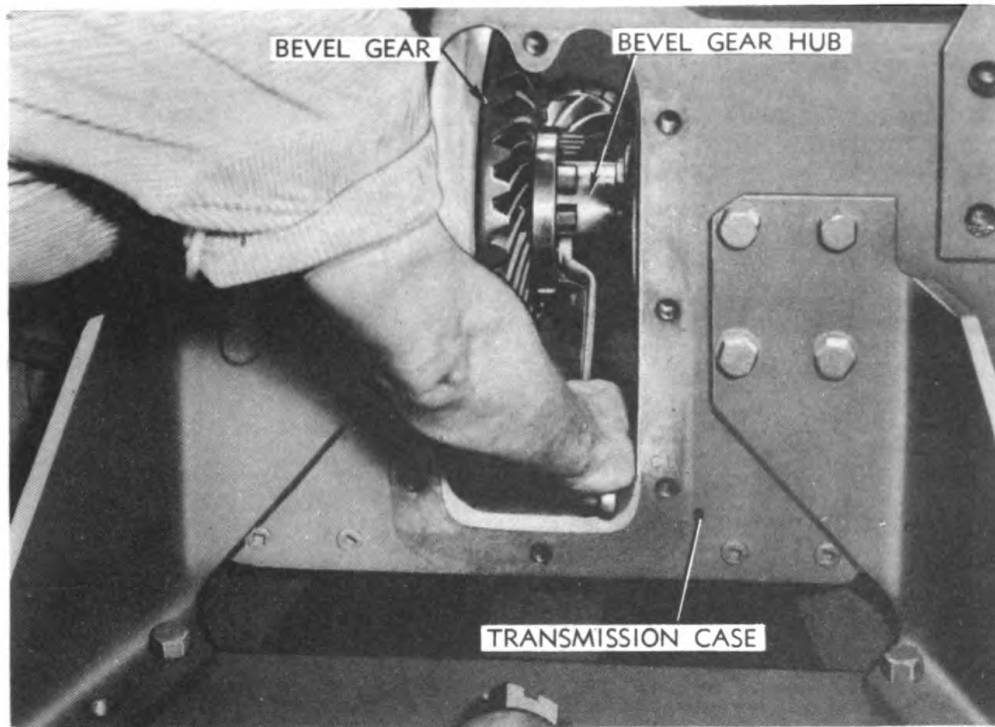
Figure 165 — Removing Nuts from Bevel Gear Bolts
