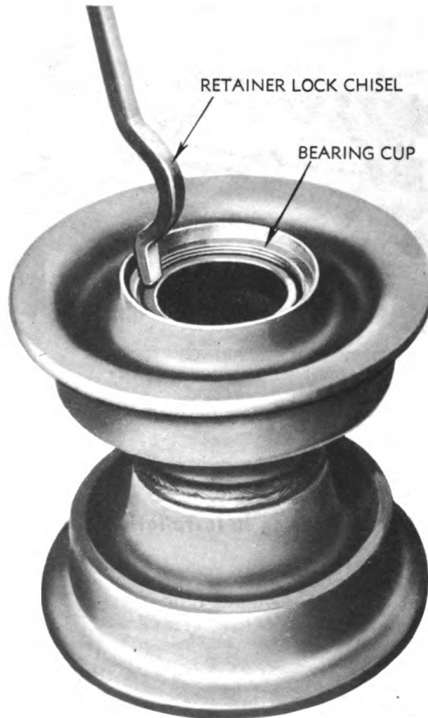
Figure 235 — Installing Bearing Cup
