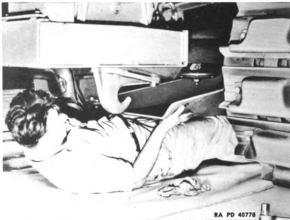
Figure 282 — Removing Engine Support Bottom Cover
