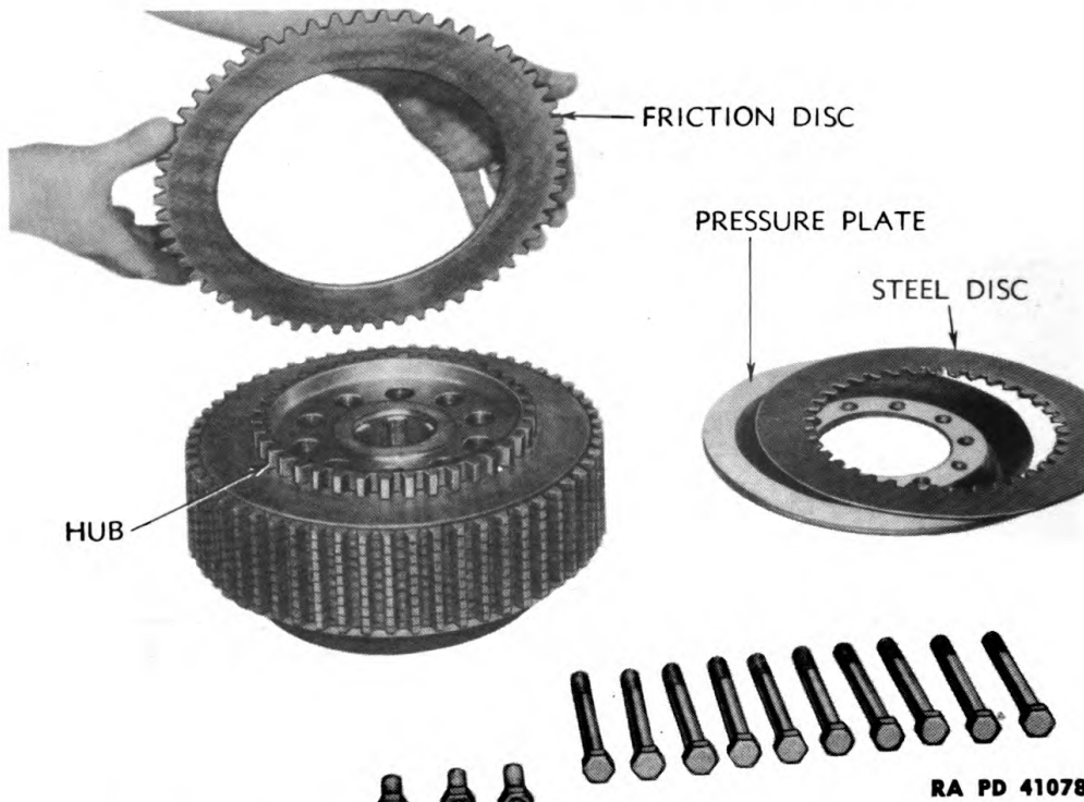
Figure 131 — Removing Friction Disk from Hub
