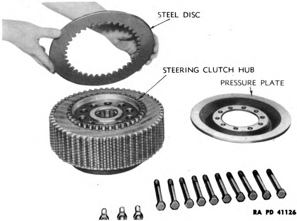
Figure 130 — Removing Steel Disk from Hub
