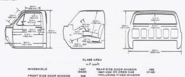
Note: Interior dimensions measured with front seat in rearmost position; seat travel is 5 inches.
