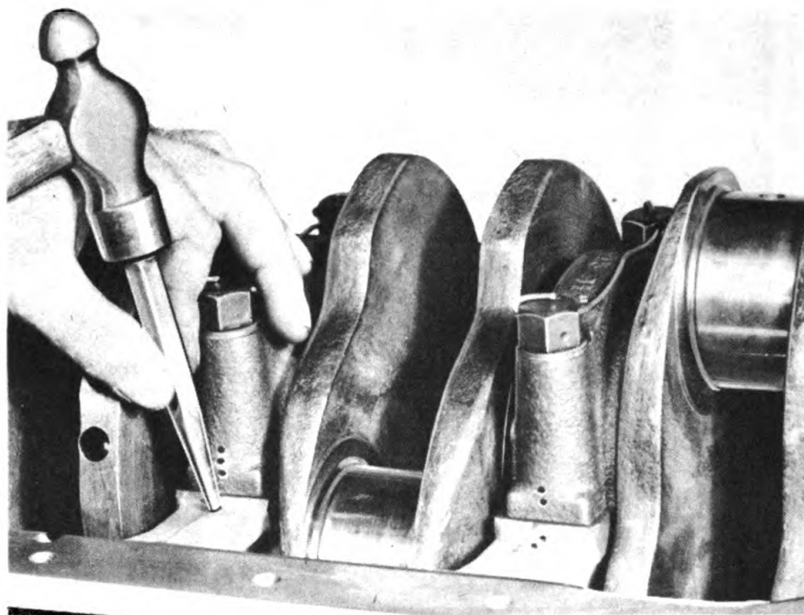
Figure 19 — Marking Identification of Main Bearing Caps
