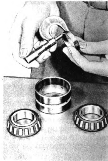
Measuring Spacer With Micrometer Calipers (41-C-307)
