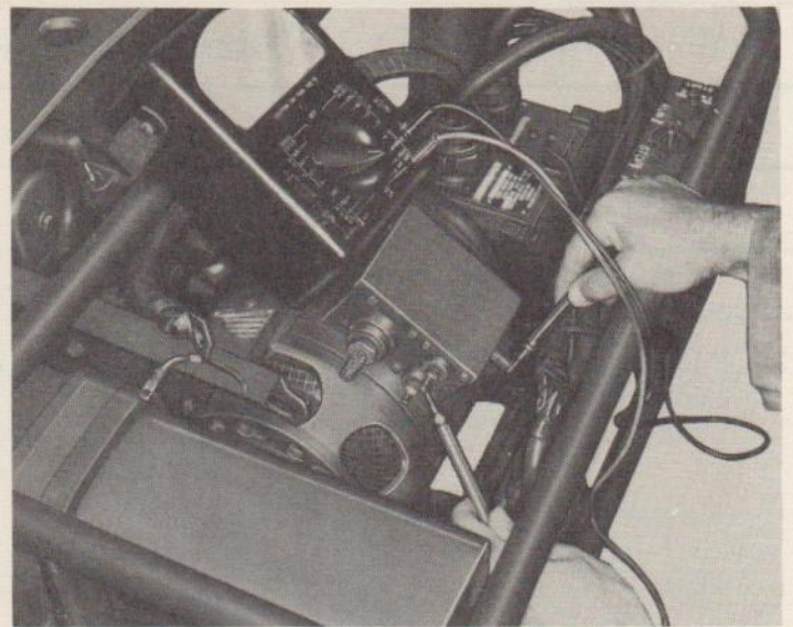
B. Place ohmmeter prods on terminals D and E. If ohmmeter reads zero or infinity, notify higher echelon.
