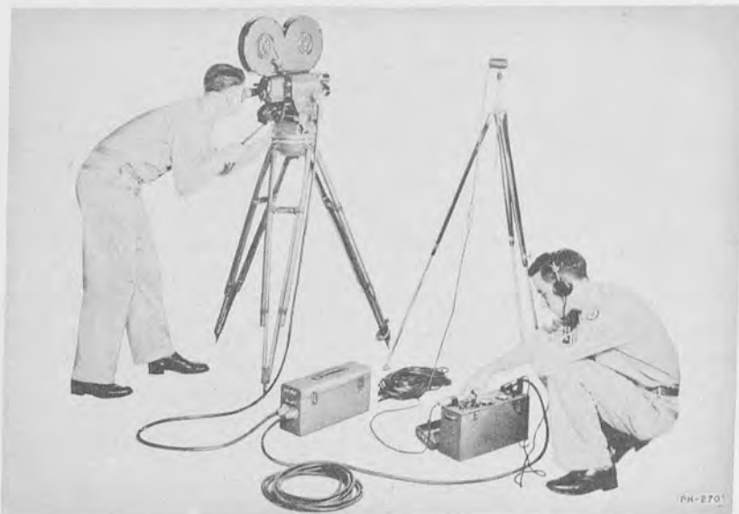
Figure 66. Camera PH-270, in use with Recorder PH-271.
