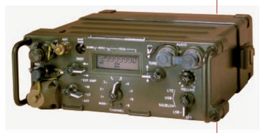
Datron's PRC1099A is an HF/SSB tactical manpack transceiver designed for demanding battlefield applications. It is a 20W radio operating over the full 1.6 - 30 MHz frequency range with 10 Hz resolution. The PRC1099A is rugged, lightweight, easy to use, and can be configured with numerous add-on ancillaries and accessories to create a wide variety of manpack, mobile, or base station systems.
