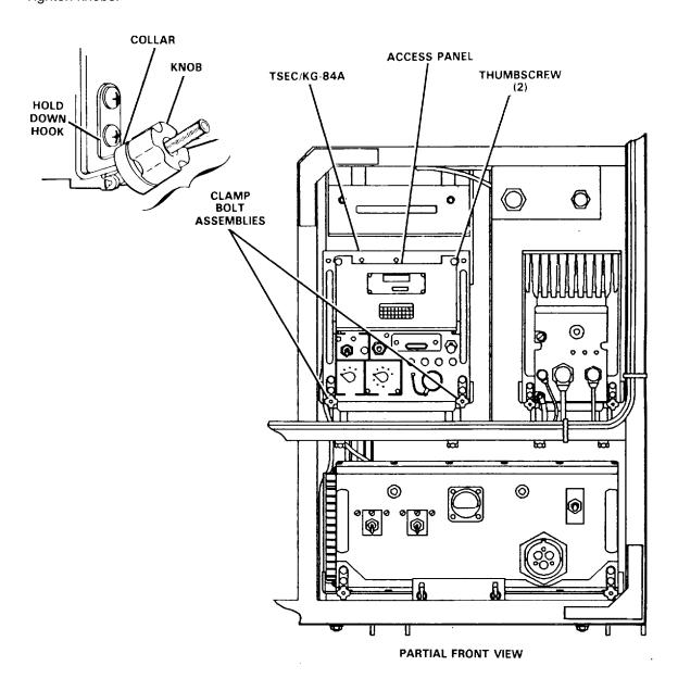
(3) KG-84 Nonsecure Bypass Assembly Hookup. The KG-84 nonsecure bypass assembly is utilized during nonsecure data operations (with TSEC/KG-84A removed).
