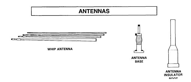
Antenna Assembly AS-3809/G (Whip Antenna) has a frequency range of 2.00 to 29.99 MHz. It consists of four 4-foot sections and Base, Antenna AB-1335/G (Antenna Base). The antenna insulator boot (not part of the Whip Antenna) fits over the Antenna Base to protect personnel from direct contact with the Whip Antenna and possible serious injury.
