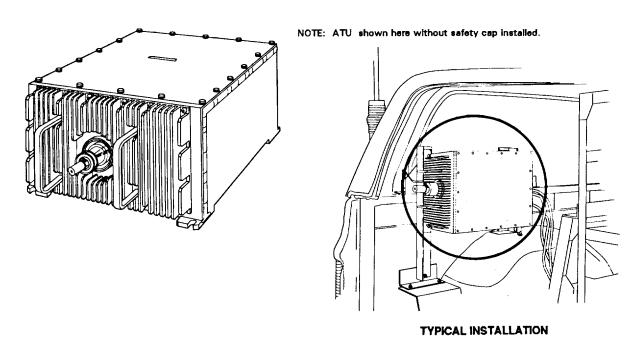
The ATU mounts separately on the selected vehicle. The ATU provides'the impedance matching between the antenna and the PA. Functional capabilities include:
