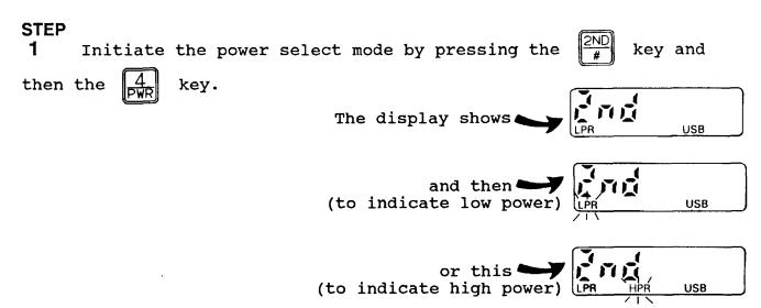
The power level indicator blinks to show the present power setting of the Manpack.
