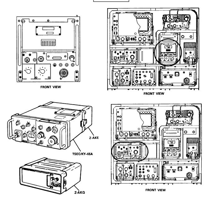
The TSEC/KY-65Aencrypts and decrypts voice traffic. AC/DC Power Supply Z-AKE powers TSEC/KY-65Awhen in the vehicular configuration. Battery Pack Assembly Z-AKG powers TSEC/KY-65Awhen in the manpack configuration.
