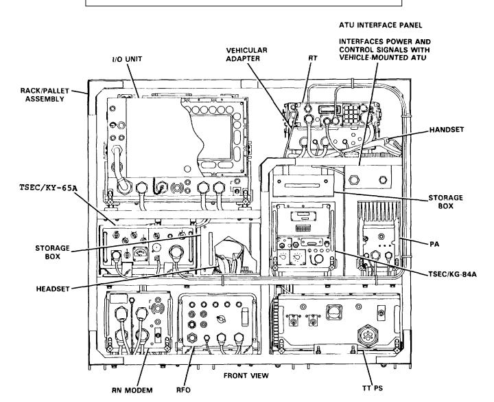
All operating components except the ATU, Remote Control Set, and antennas are housed in a rack/pallet assembly (rack). The rack is normally installed in a vehicle. The COMSEC equipments, TSEC/KG-84A andTSEC/KY-65A, are furnished separately.
