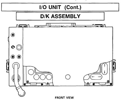
The D/K assembly provides operator interface. It displays menus in response to operational sequences. The D/K assembly is also used to compose and view messages, perform network communications and for initiating BIT.
