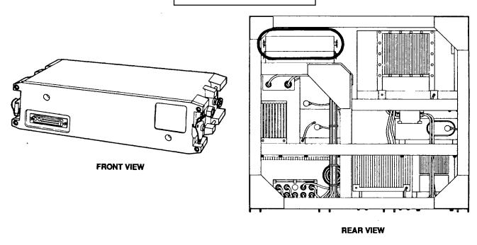
The Battery Case/Charger provides dc power for the RT when in the Manpack configuration.
