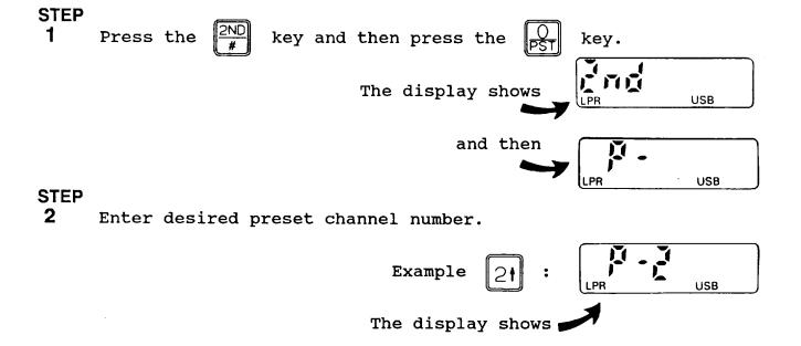
Each time a number key is pressed, the display shows the number of the preset channel.
