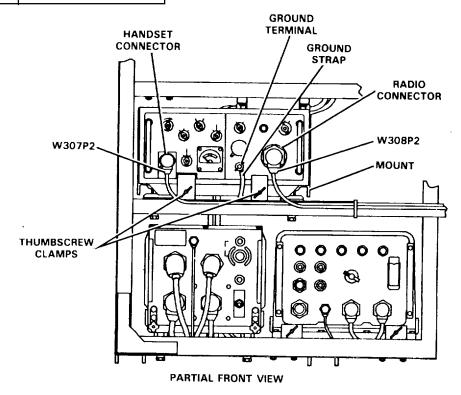
(2) Installation of TSEC/KG-84A. Preparation of the TSEC/KG-84A must be made with the assistance of unit or higher level maintenance.
