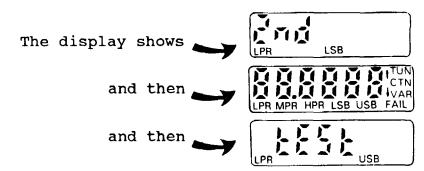
(2) Upon successful completion of BIT, the RT display shows the frequency setting now in memory.
