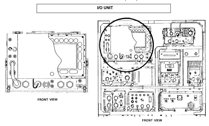
The I/O Unit provides the capability to transmit and receive Regency Net messages. It manages, maintains and controls the operating modes of the Team Terminal. The I/O Unit consists of a removable display/keypad (D/K) assembly and the controller assembly. These assemblies are connected by the remote cable to allow the D/K assembly to be mounted in the rack with the controller assembly or mounted separately (via a 20-foot remote cable) in a position more convenient to the operator.
