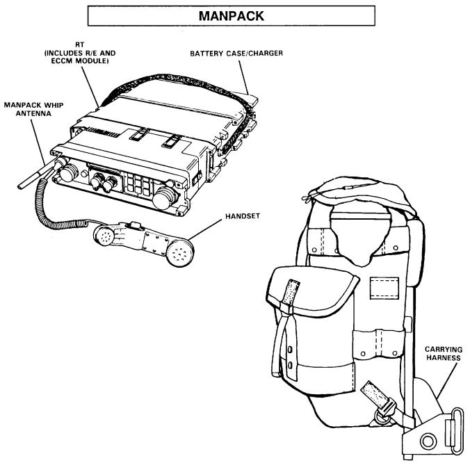
The Manpack provides single channel HF secure or nonsecure voice communications. It enables the Team Terminal operator to leave the vehicle and maintain voice communications at reduced power. The Manpack is assembled using the RT (comprised of R/E and ECCM Module), Battery Case/Charger, Manpack Whip Antenna, Handset and carrying harness. When in the secure mode, the TSEC/KY-65 is removed from the rack and connected to the Manpack via hard-wire.
