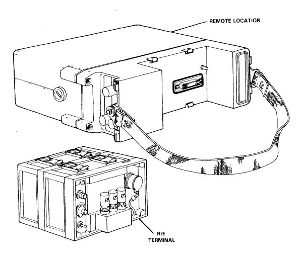
The Remote Control Set provides remote operation of the Team Terminal. It consists of the R/E terminal and the remote location. When deployed, the R/E terminal is interchanged with the ECCM Module of the RT and then the R/E terminal and remote location are connected via field wire.
