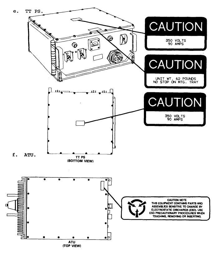
NOTE: ATU shown here without Safety Cap or Matching Capacitor installed.
