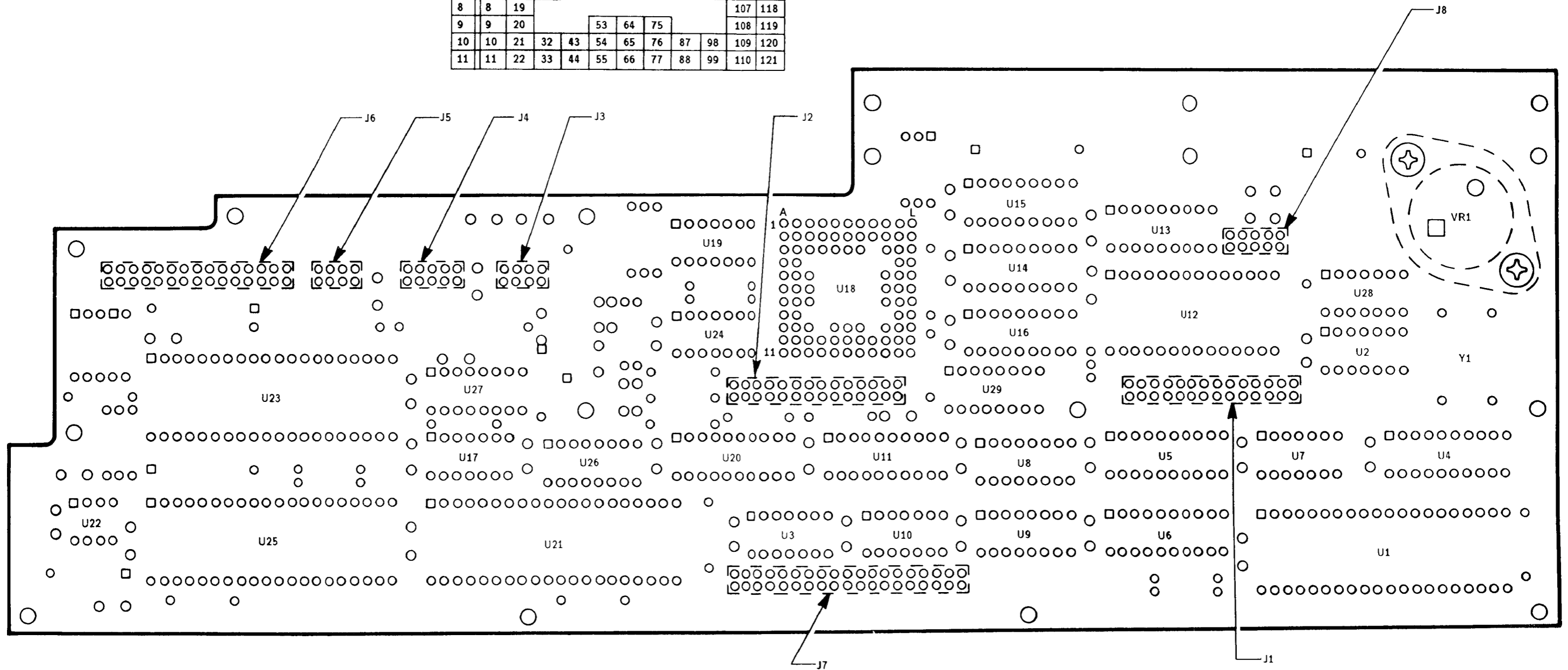
Figure B-5b AM/RC Circuit Card Assembly Solder Side
