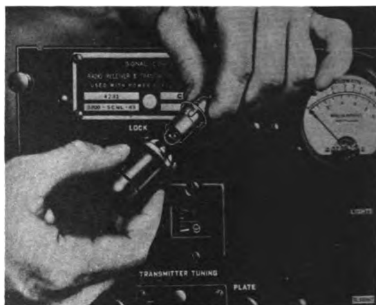
Figure 87. Meter pilot light removed from housing.
