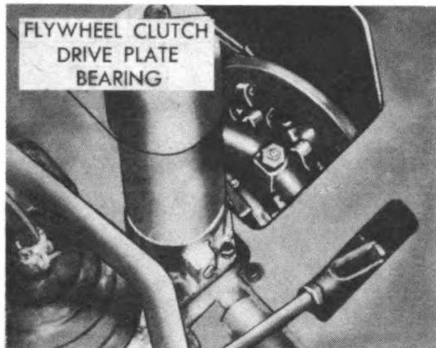
Ref. 41: Lubricate bearings sparingly every day. Turn clutch shaft until fitting appears.
