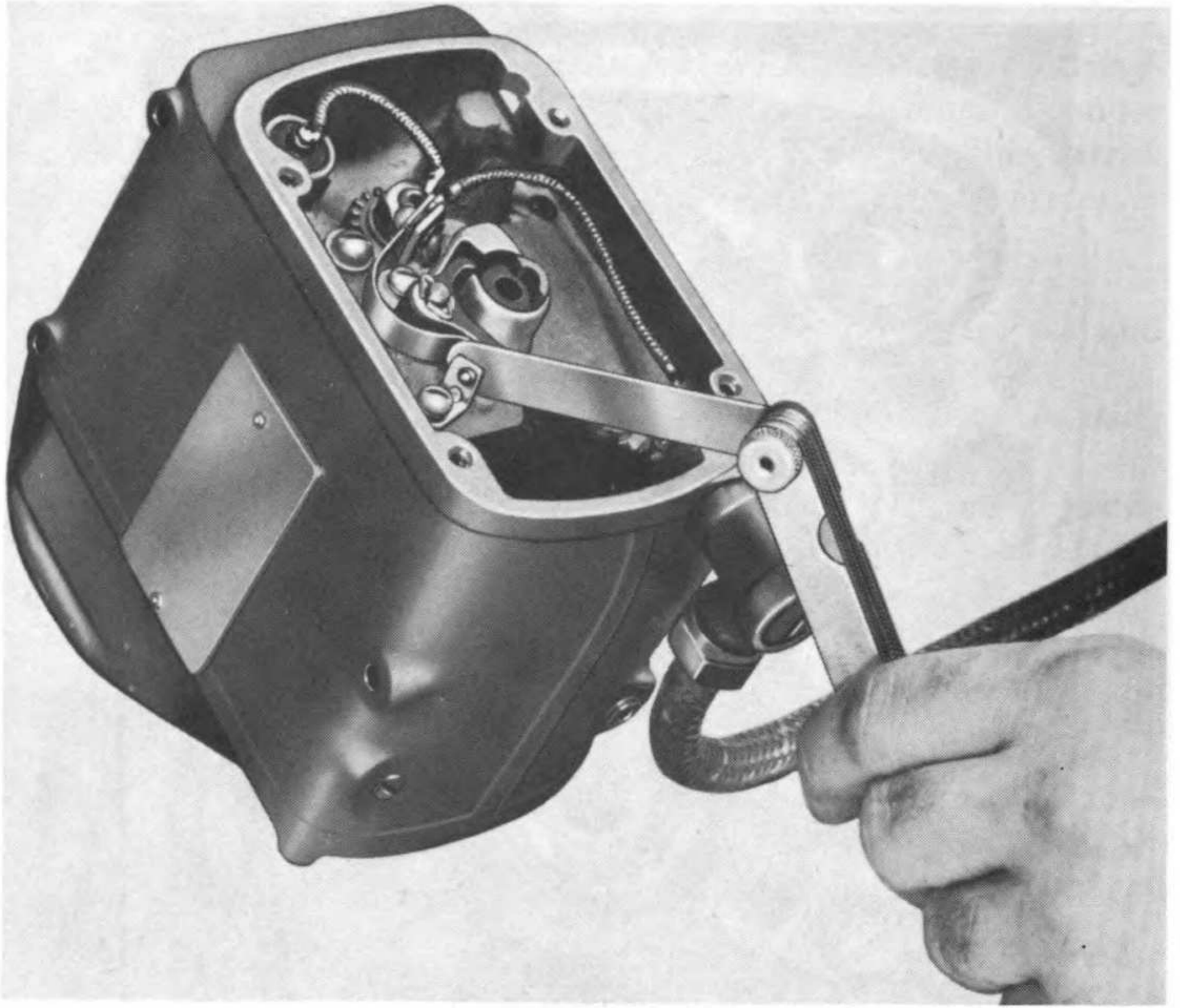
Figure 43. Checking contact point opening.
