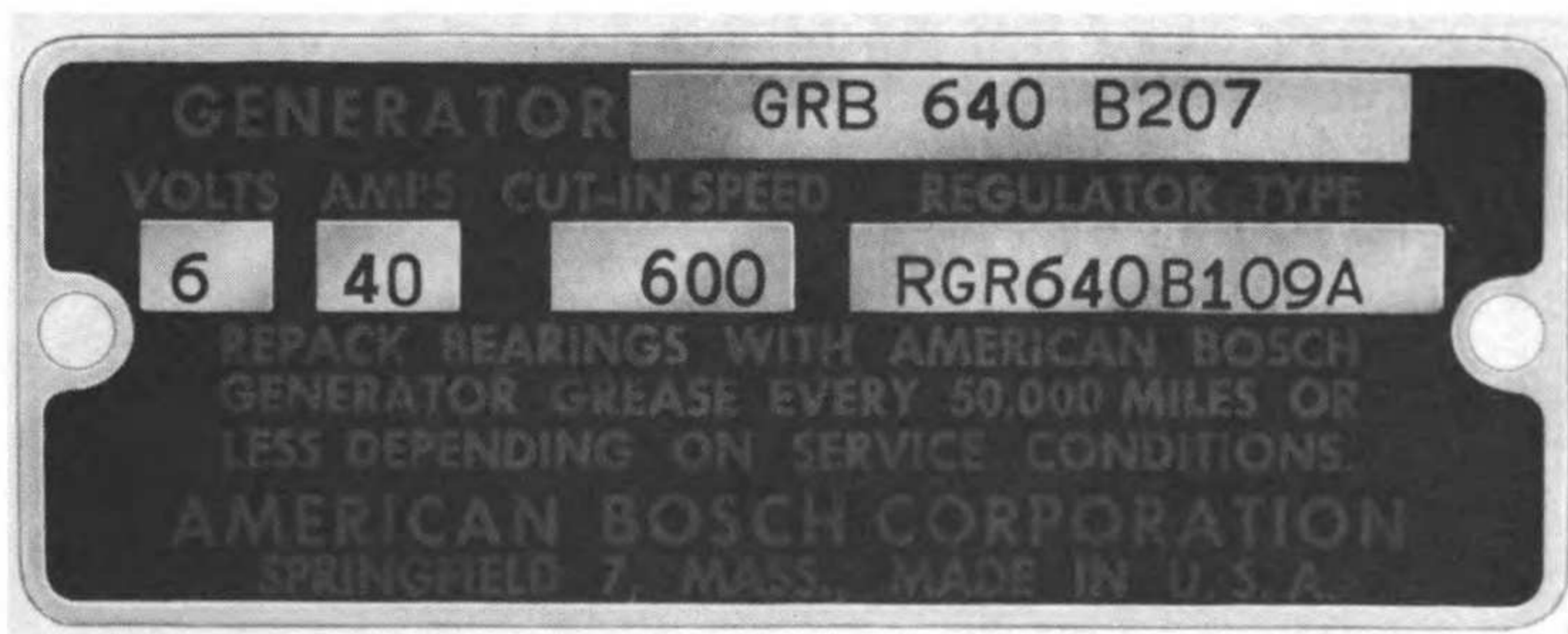
Figure 8. Generator serial number.
