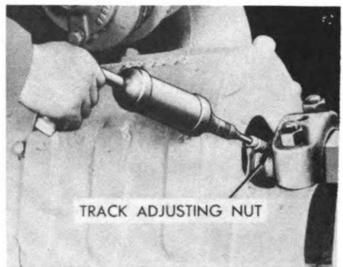
Ref. 42: When equipped with fittings, lubricate monthly. Remove plates on both sides of tractor to make fittings accessible.
