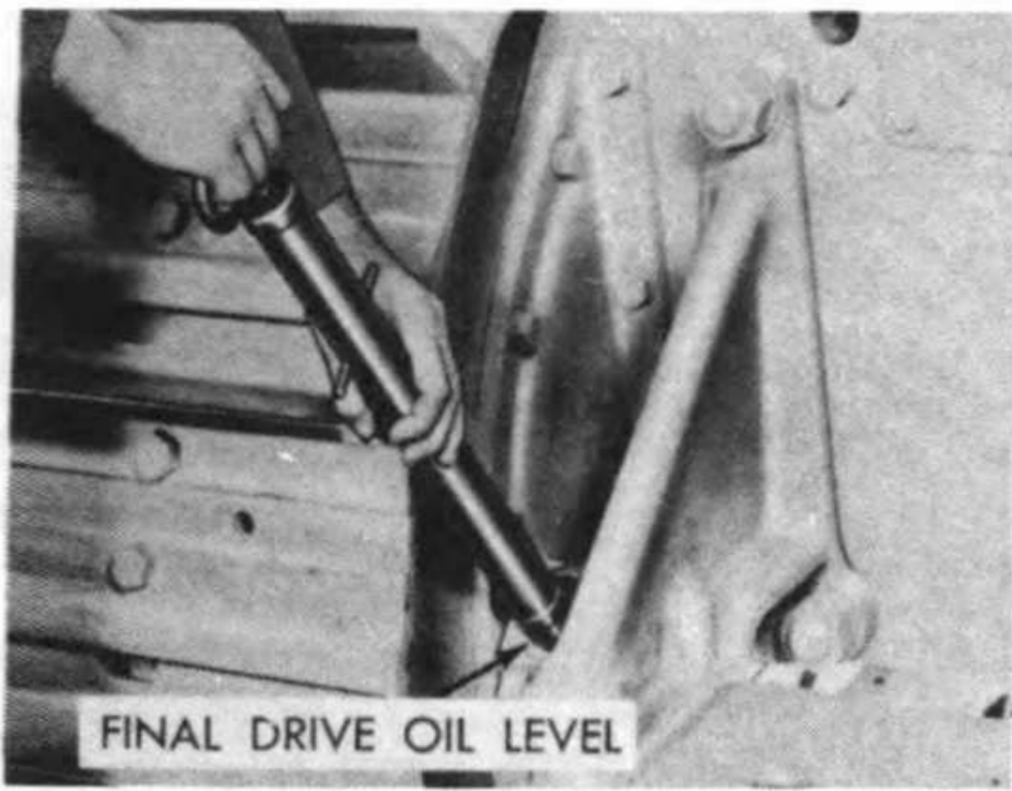
Ref. 43: Check oil level by removing two filler plugs, one for each side, every week. Keep lubricant to level of filler openings.
