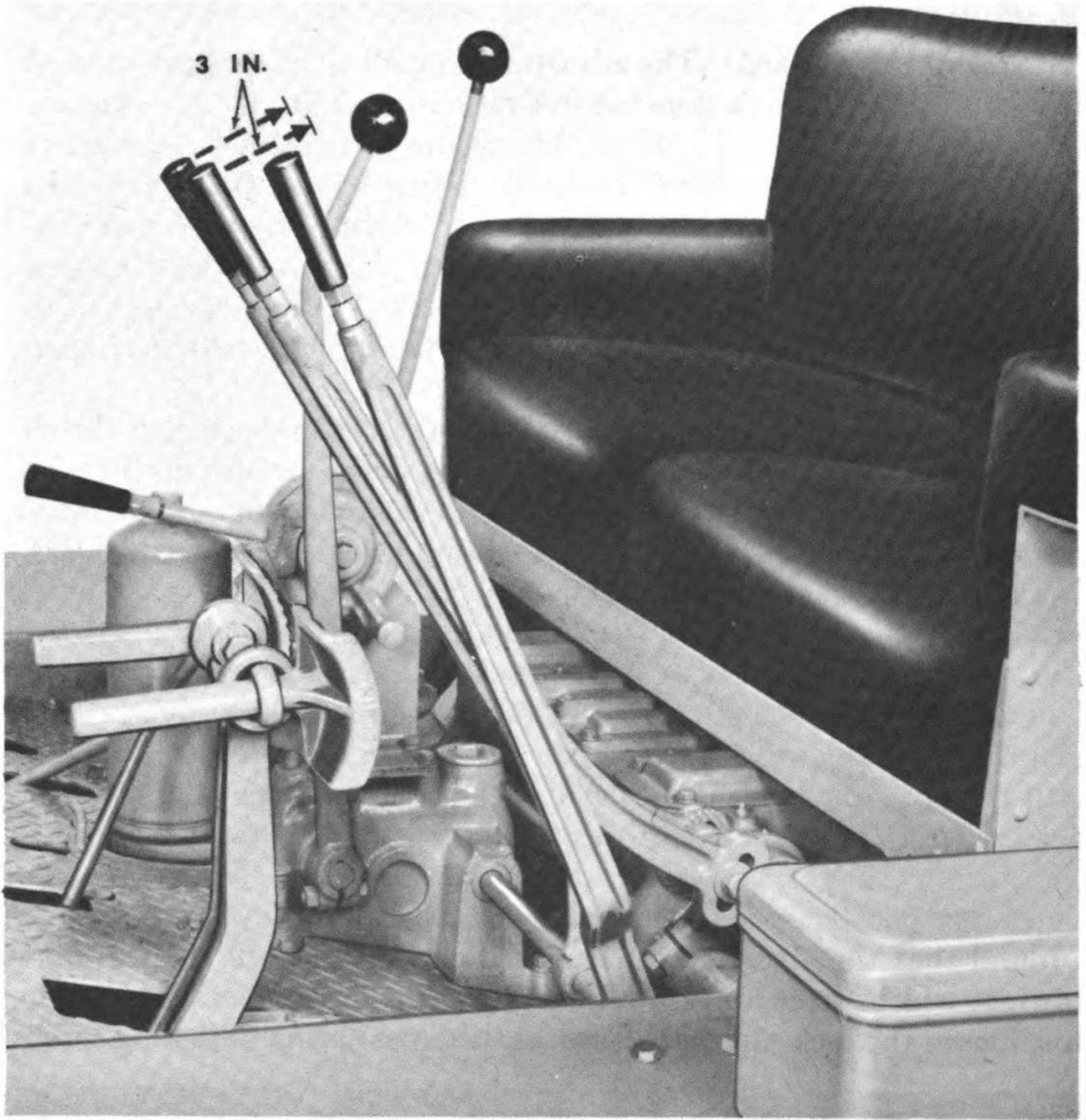
Figure 92. Steering clutch control lever free movement.
