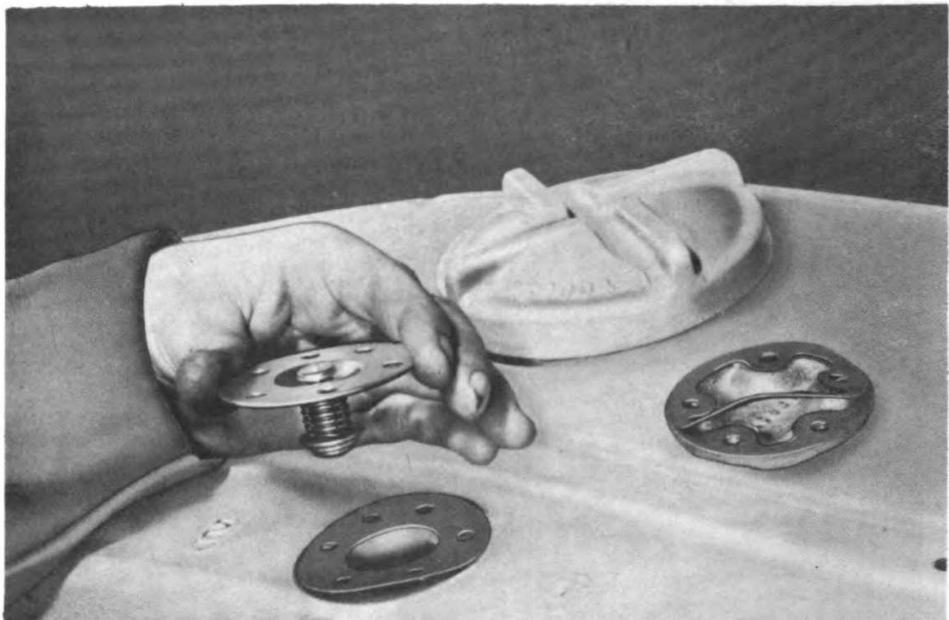
Figure 65. Removing sealed pressure overflow valve.
