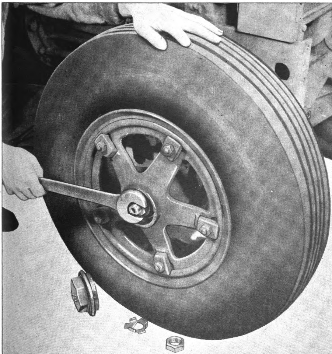
Fig. 92. Adjusting Front Wheel Bearing
