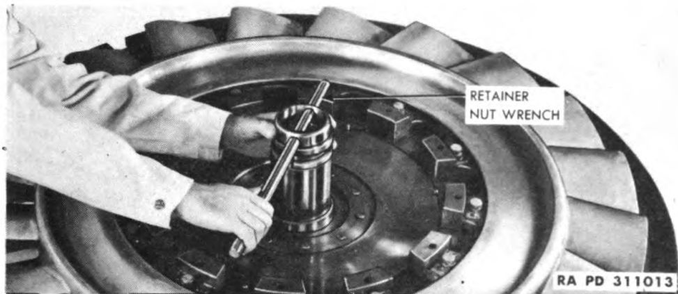
Figure 8 — Loosening Flywheel Retaining Nut, Using Wrench 5A2303
