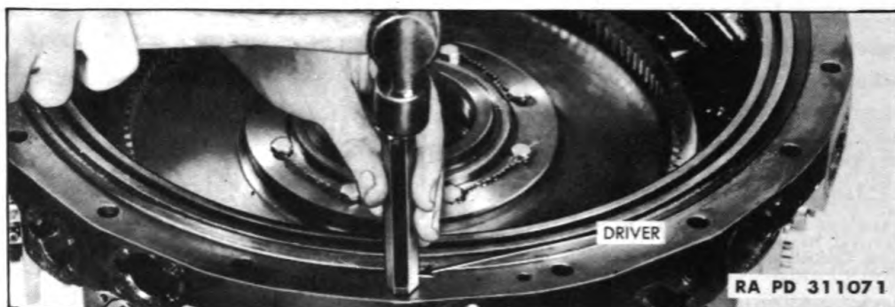
Figure 33 — Installing Fuel Pump Sleeve, Using Driver 5A2171
