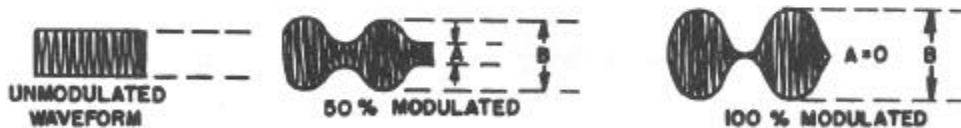
Figure 7-18—Wave Envelope Method of Checking Modulation
