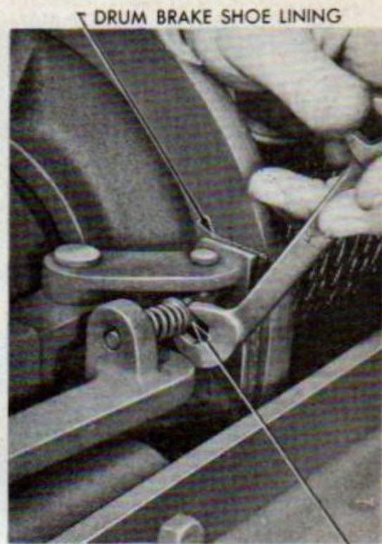
SHOE ADJUSTING AND LOCK NUTS RA PD 53084
