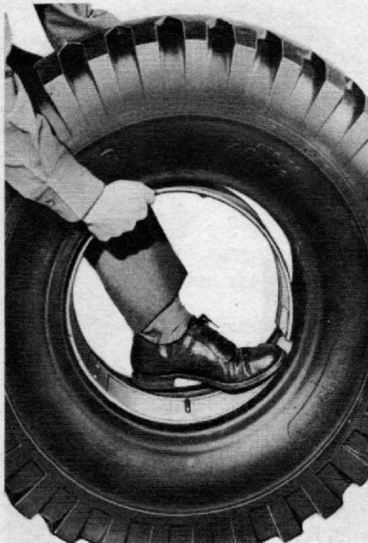
EXPANDING TIRE BEAD LOCK RING IN TIRE
