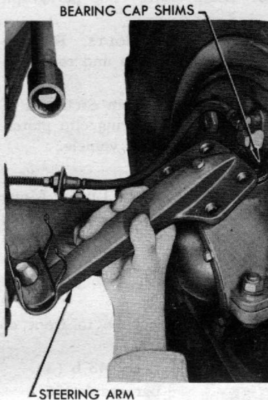
Figure 133 — Removing Steering Arm
