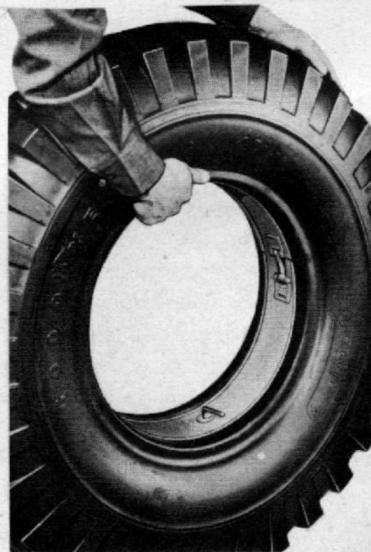
TIRE BEAD LOCK RING INSTALLED
