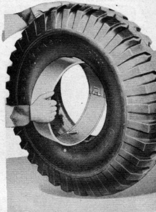
SLIDING TIRE BEAD LOCK RING ON VALVE STEM
