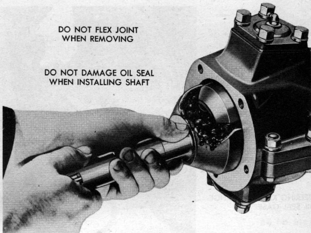
Figure 129 — Removing Universal Drive Assembly
