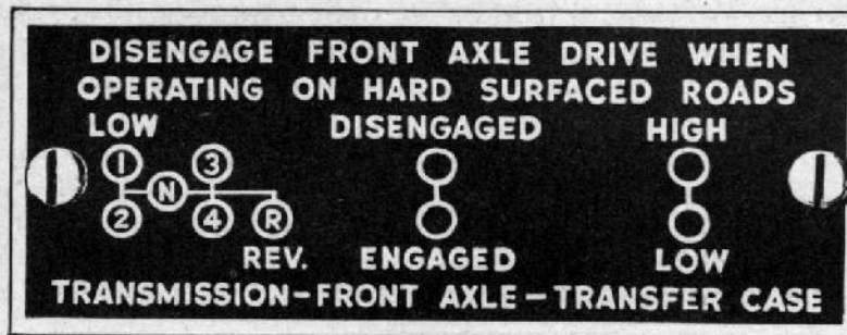
Figure 13 — Speed Caution Plate
