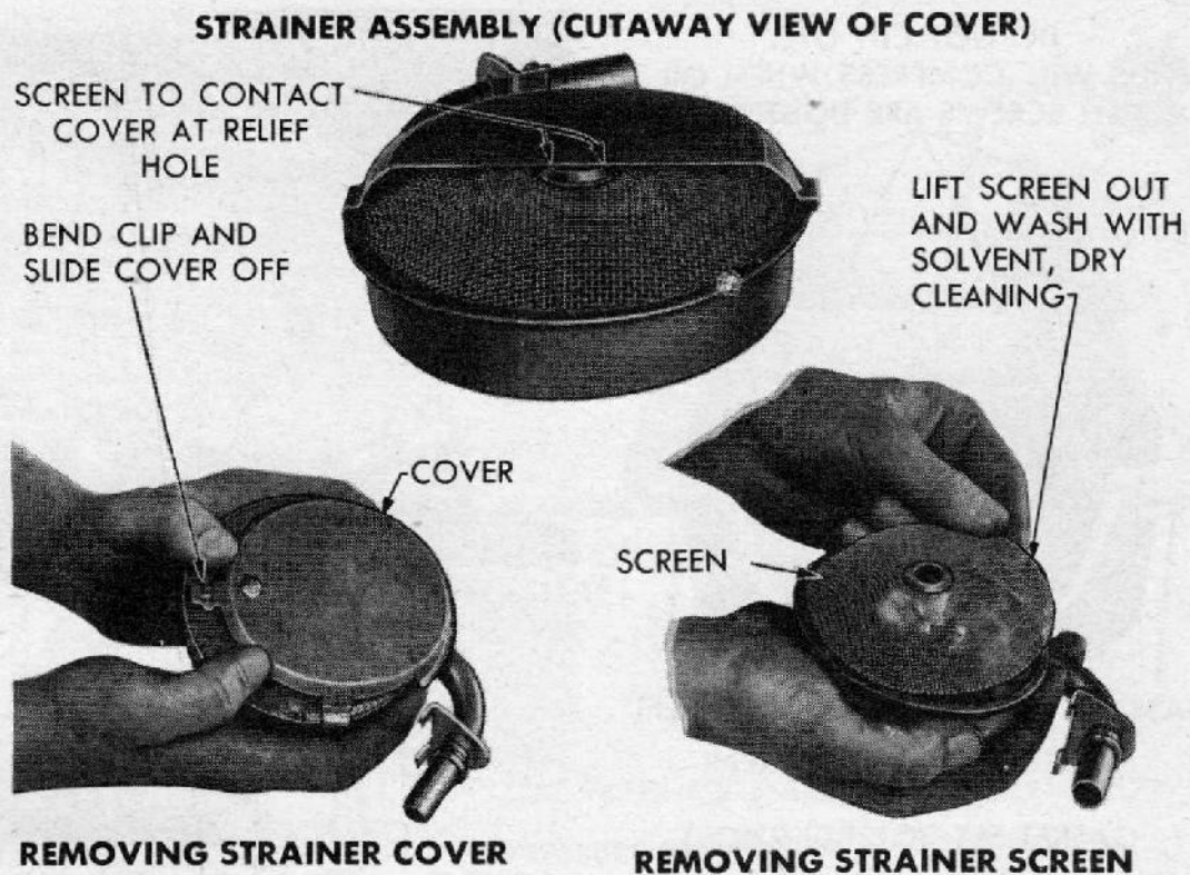
Figure 46 – Oil Strainer
