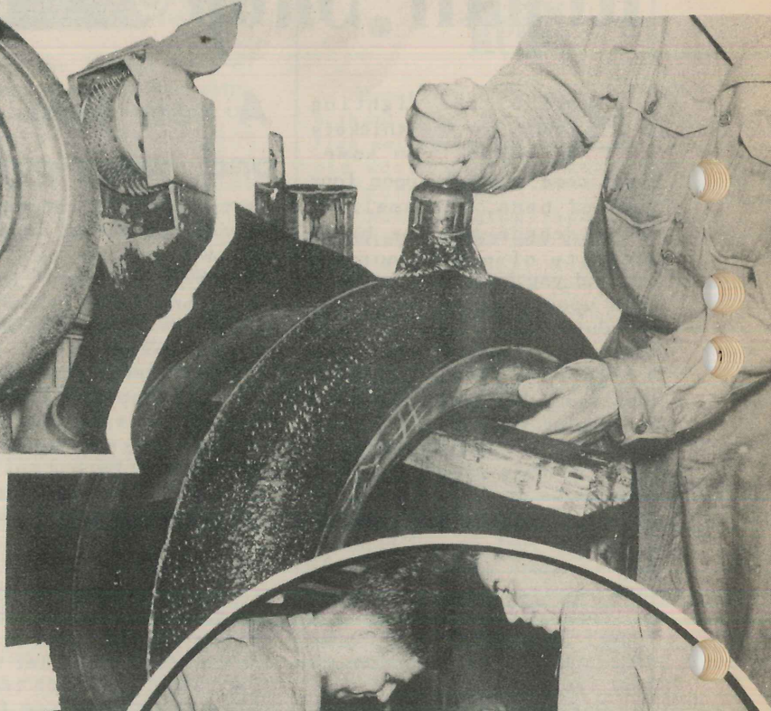
1 'Buffing.' As little rubber as possible is roughed off. The buffed surface guarantees a good bond between the old carcass and the retread.
