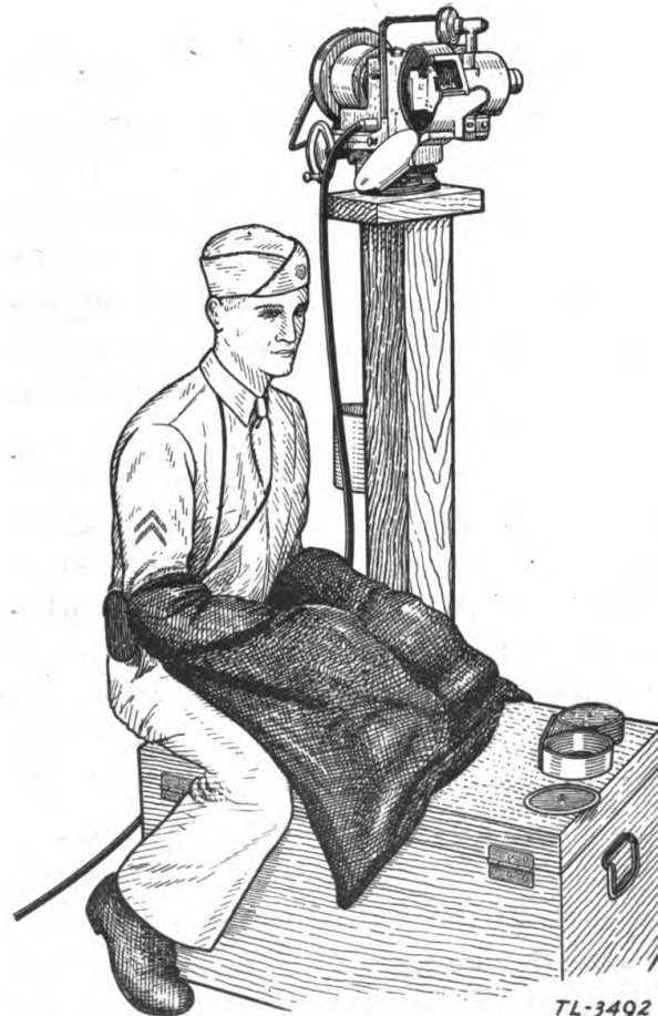
FIGURE 18.—Soldier loading film magazine with changing bag.
