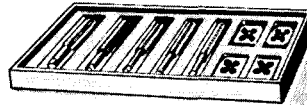
RIGHT—HAVE AN ARRANGEMENT SO TAPS AND DIES WILL NOT STRIKE EACH OTHER OR ANY OTHER TOOLS RA PD 87393
