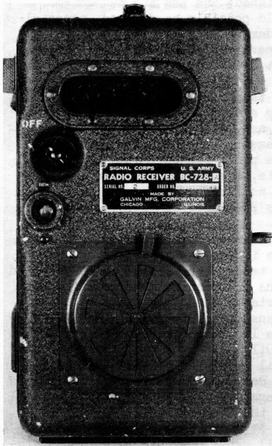
RADIO RECEIVER BC-728-( ), MAJOR COMPONENT OF THE 593. THE BLAST PROTECTOR IS SHOWN IN CLOSED POSITION
