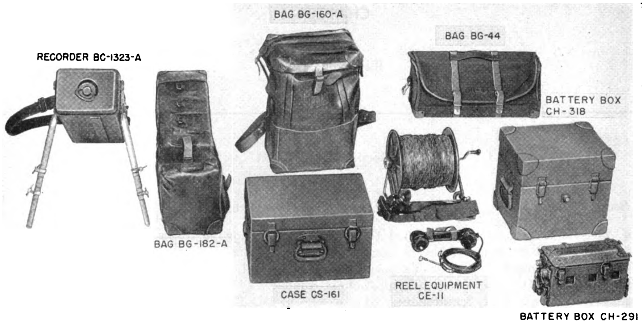
Figure 2. Sound Locating Set GR-6-A, major components.
