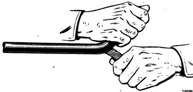
Figure 4. Method of separating rubber jacket from conductor.
