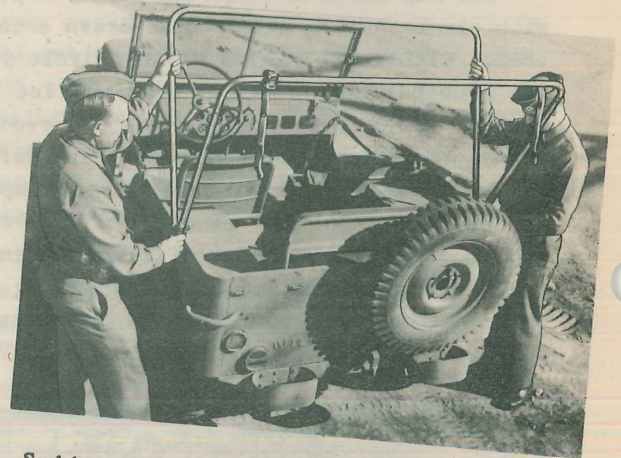
Soldiers pull frame upright and fasten in socket with same wing nut. Rain drizzles steadily.
