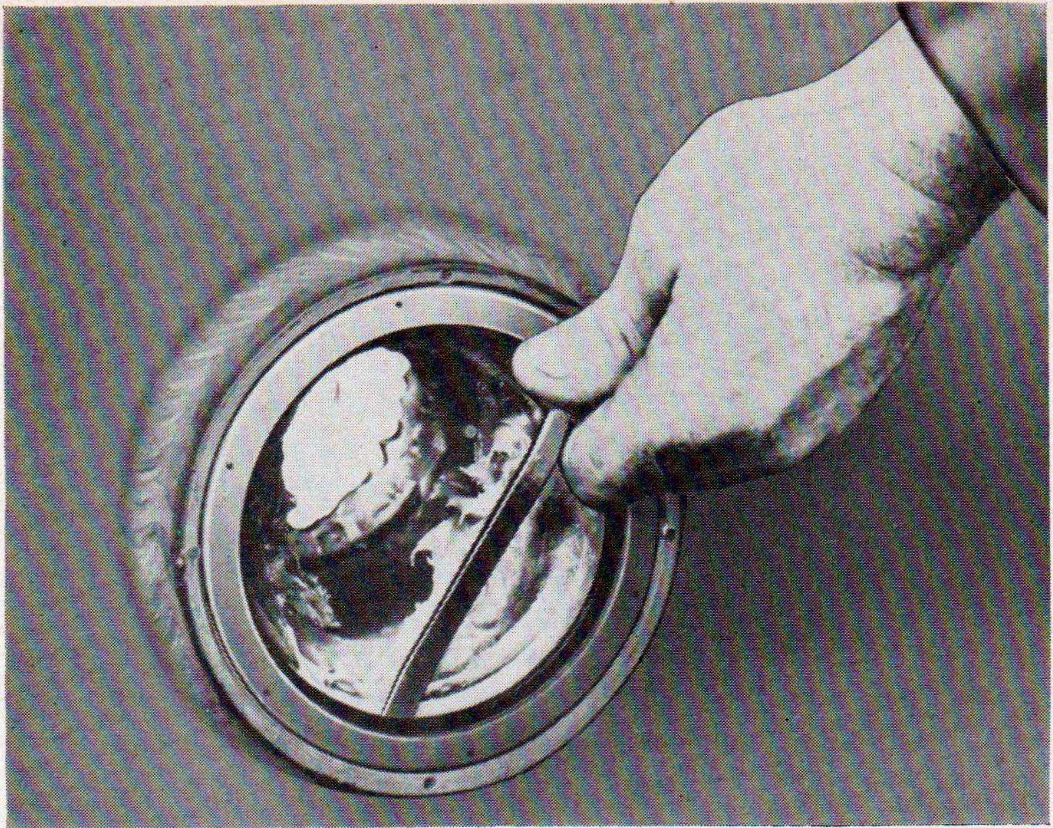
Figure 22. Removing oil seal.
