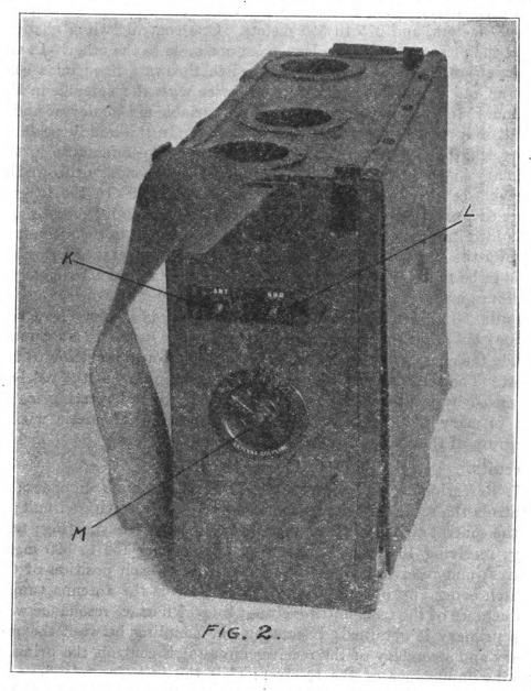
able in six steps controlled by one switch known as a "wave-change" switch. There is also a variable antenna tuning inductance of about 11½ turns in the secondary so that it can be exactly adjusted to resonance with the primary. A coupling switch controls the amount of inductance common to both the primary and secondary, and thus allows the coupling to be varied. The minimum coupling is at "1"
