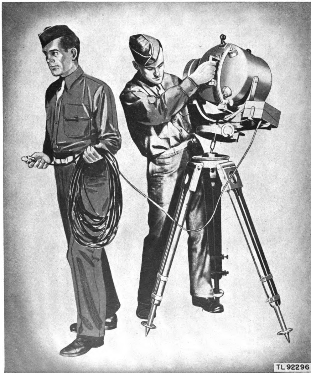
Figure 9. Placing signal lamp on Tripod LG-9.
