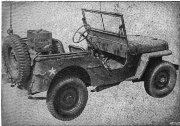
Figure 2. Radio Set SCR-610-( ), ground vehicular installation.
