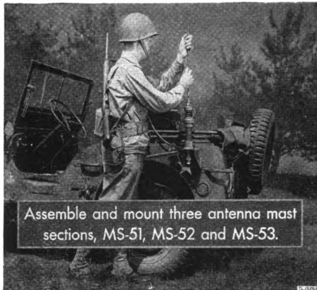
Figure 39. Radio Set SCR-610-( ), assembling and mounting of Mast Sections MS-51, MS-52, and MS-53.
