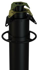
Will-Burt's Quick Erecting Antenna Mast (QEAM) is a series of reliable screw-drive or strap-drive guyed field masts made of high-strength 6061-T6 aluminum tubes. The HDTM 10C and the TM 15C are made from carbon composite tubes. Designed for manual operation, QEAM elevates light payloads for ground-mounted, vehicle and shelter deployment. QEAM is an economical mast and meets MIL-STD-810 envi-
