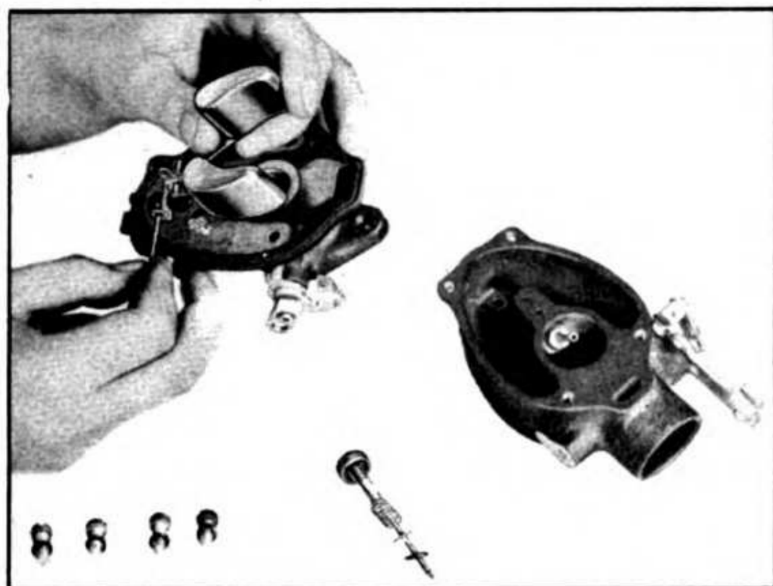
Figure 76 — Removing Carburetor Float
