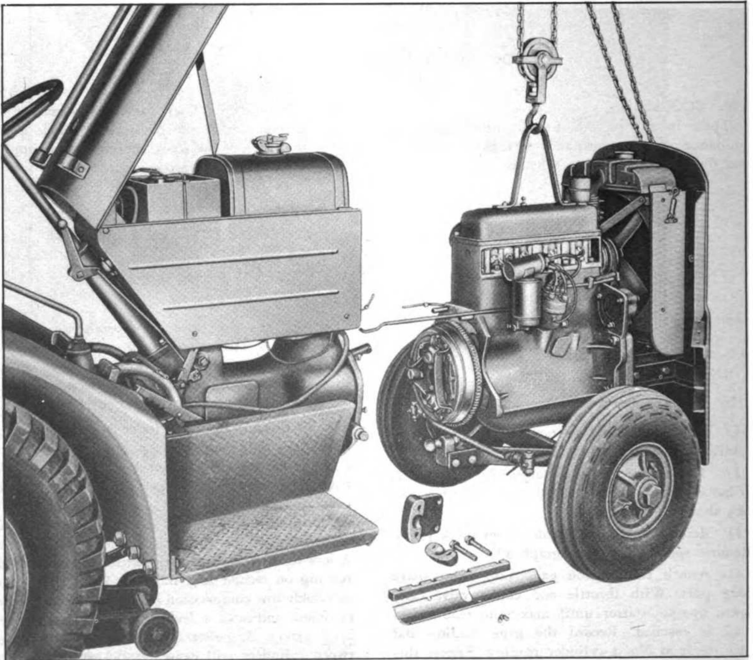
Figure 64 — Splitting Tractor Preparatory to Removing Engine
