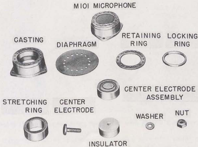
Figure 12. Microphone Assembly
