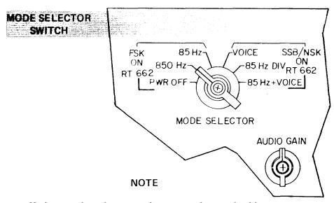
Modem mode selector settings must be used with correct service selector settings on RT-662/GRC.
