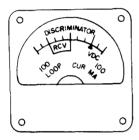
Set METER FUNCTION switch at DC LOOP NO. 2. Meter should indicate current flow of 20 or 60 mA through dc loop No. 2.
