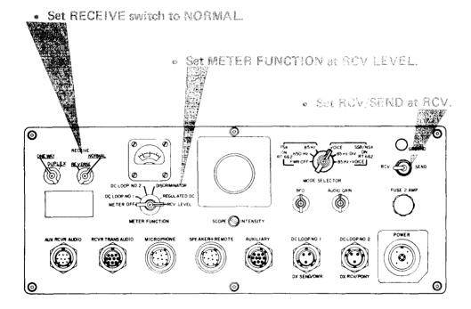
• Check ONE WAY/DUPLEX switch for ONE WAY position.
