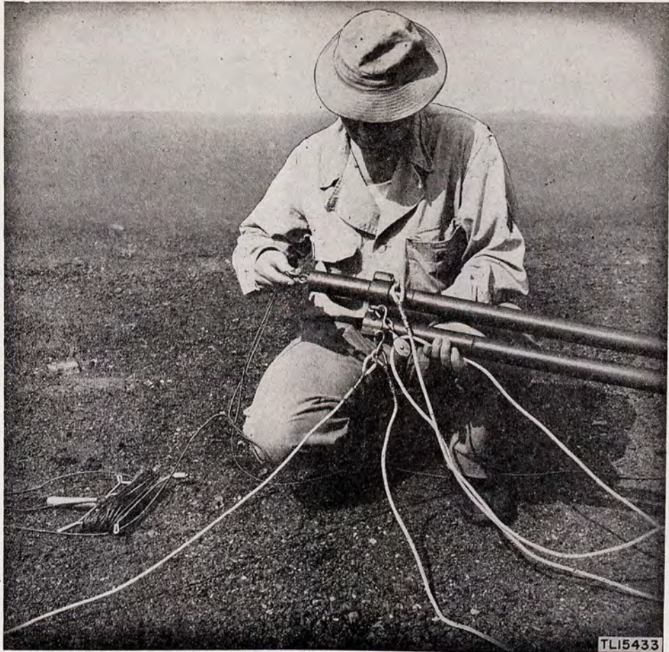
Figure 11. Antenna AN-36 being attached to Mast Section MS-91.
