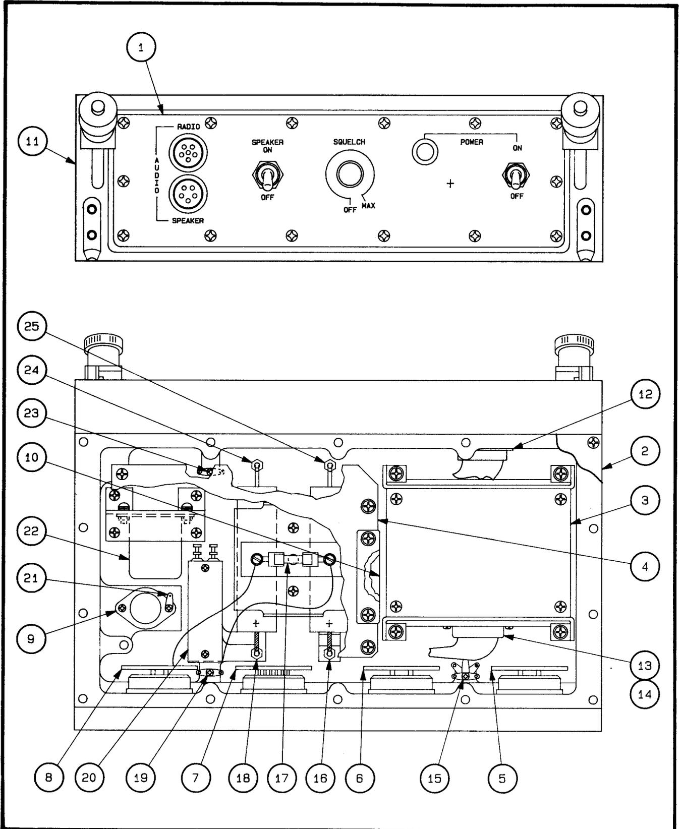
**CONTROL PANEL WIRING AND CONNECTOR MAINTENANCE INSTRUCTIONS (1 of 4)**
