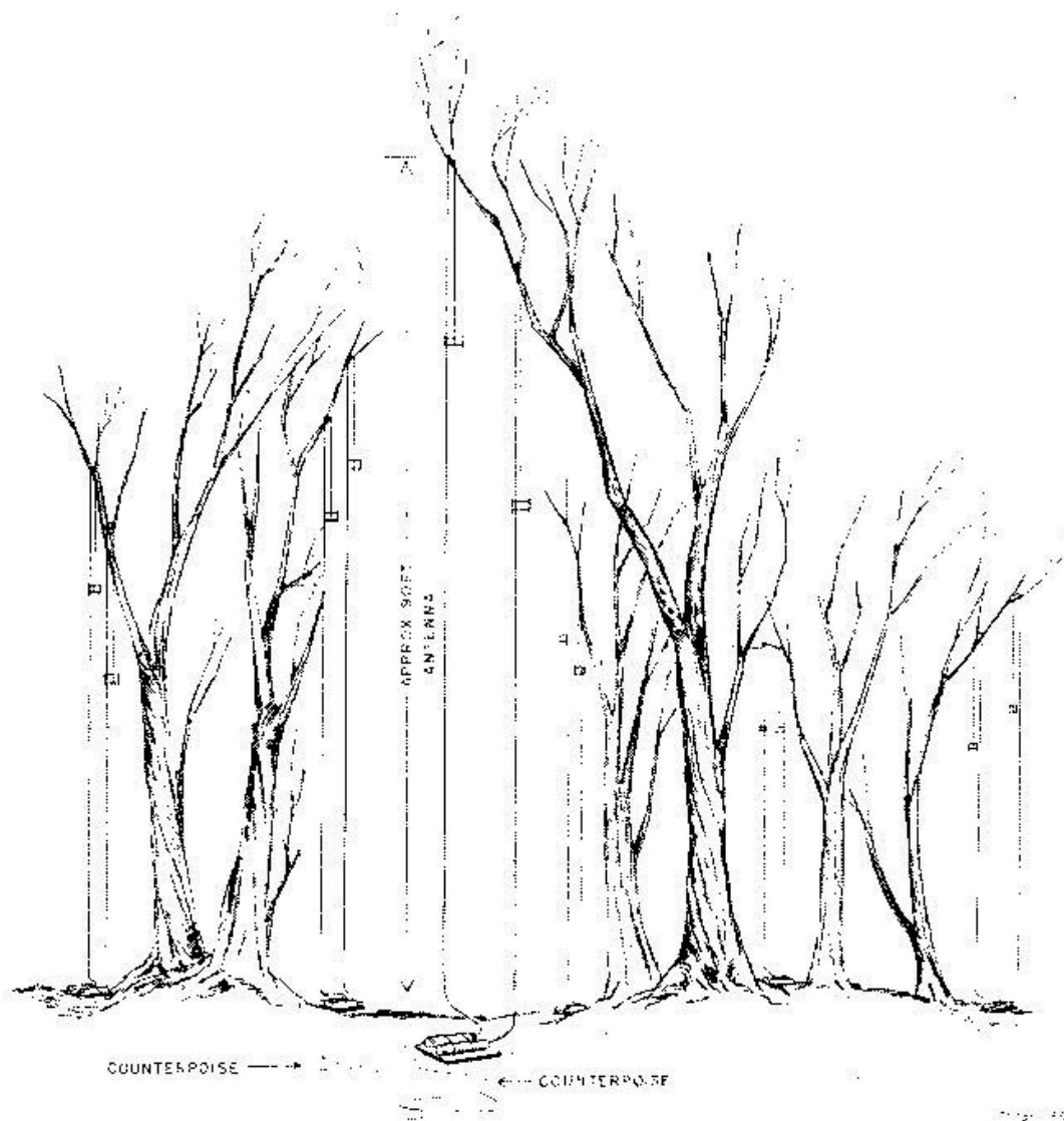
Figure 8. Vertical antenna arrangement.
