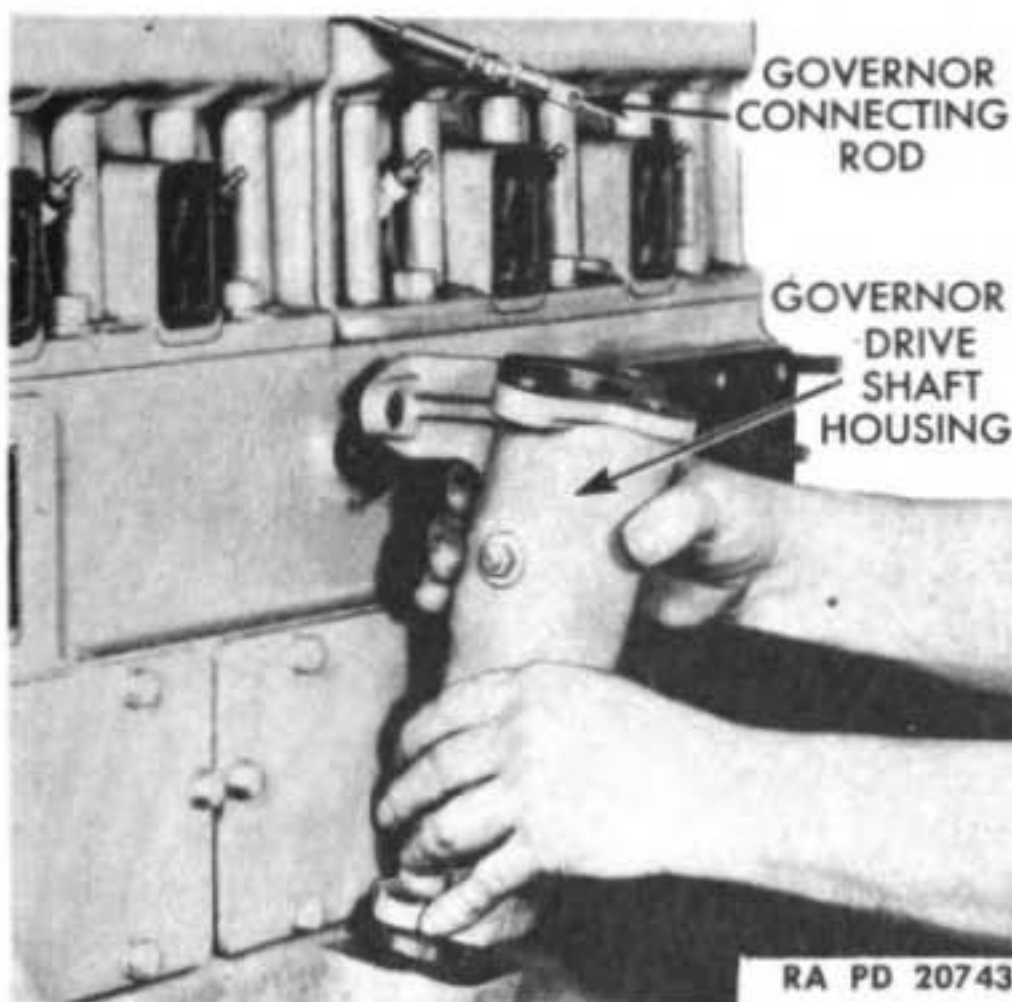
Figure 11 — Removing Governor Drive Shaft Housing
