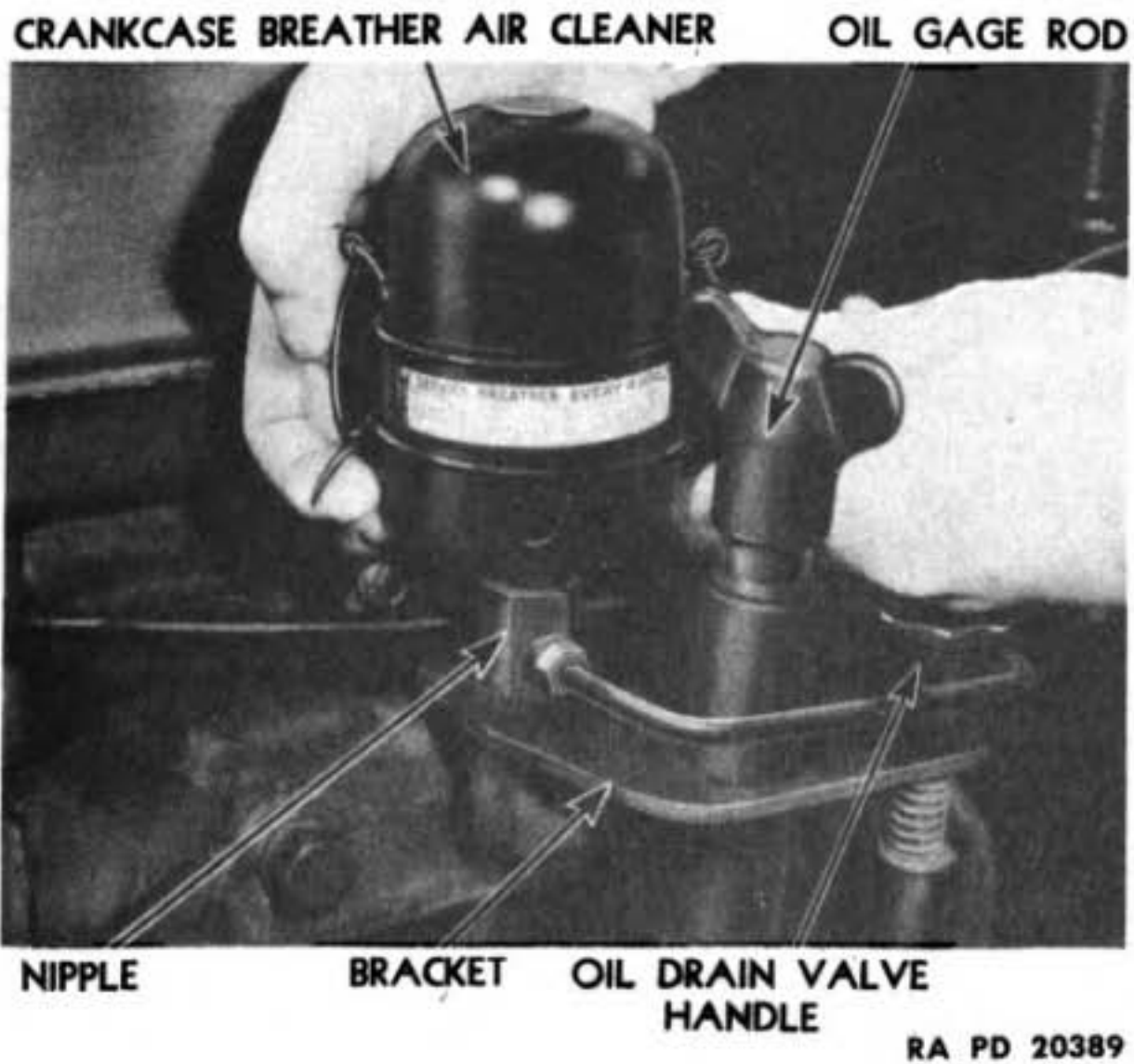
Figure 96 — Crankcase Breather Air Cleaner and Oil Gage Rod
