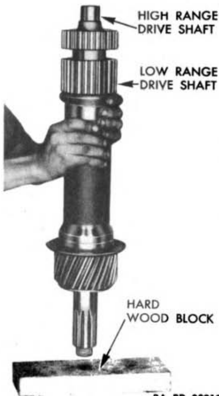
Figure 185 — Removing High-Range Drive Shaft from Low-Range Drive Shaft
