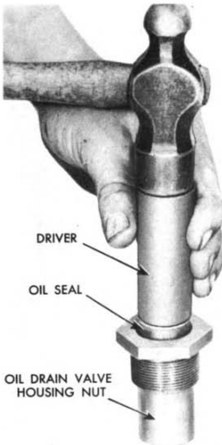
Figure 62 — Installing Oil Seal in Oil Drain Valve Housing Nut
