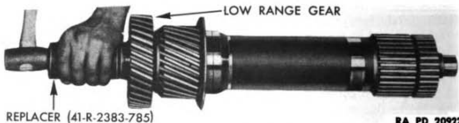
Figure 194 — Replacing Low-Range Gear with Bearing and Universal Joint Flange Clutch Low-Range Gear Replacer
