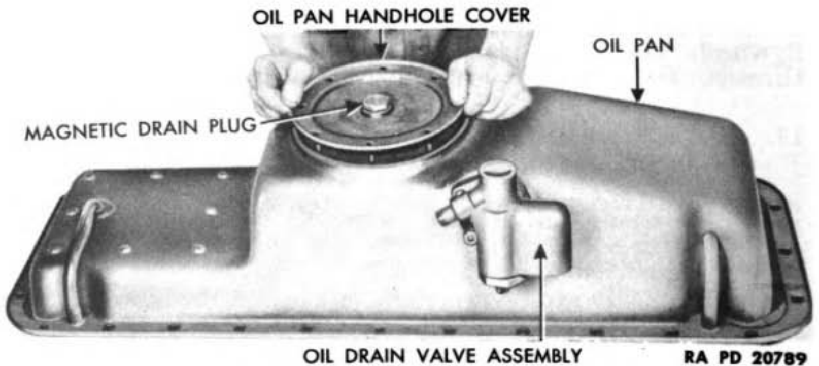
Figure 57 — Removing Oil Pan Handhole Cover
