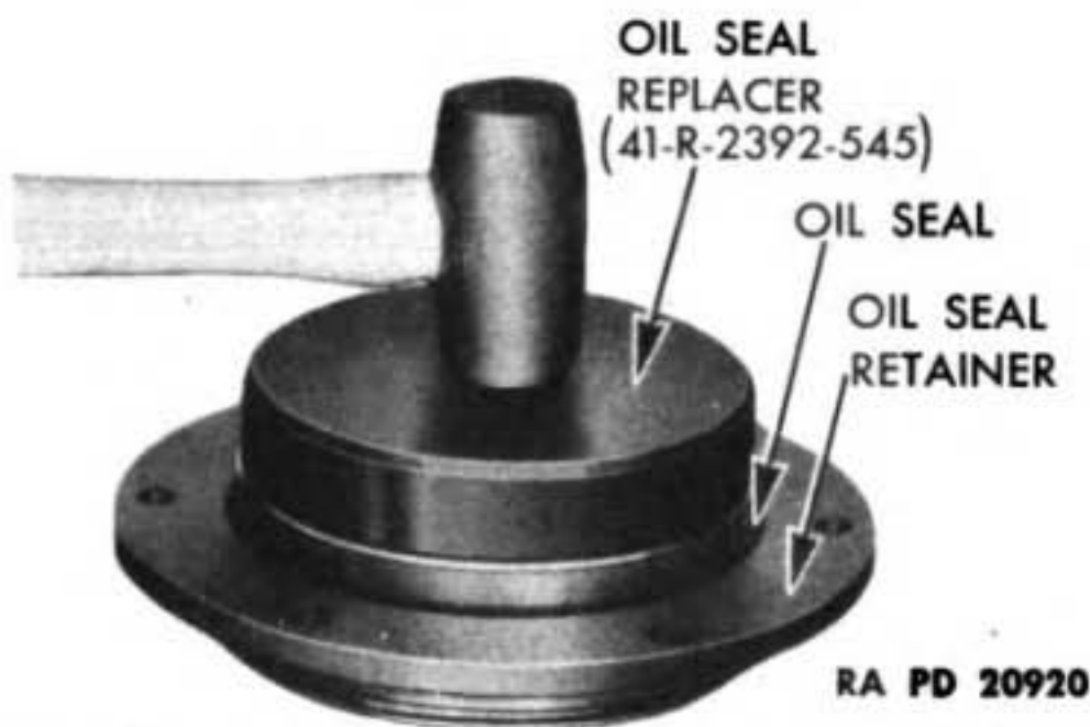
Figure 192 — Installing Low Range Drive Shaft Inner Oil Seal in Retainer with Final Drive Shaft Oil Seal Replacer
