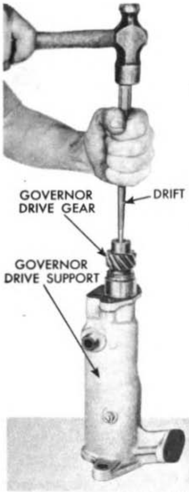
Figure 64 — Removing Governor Drive Gear
