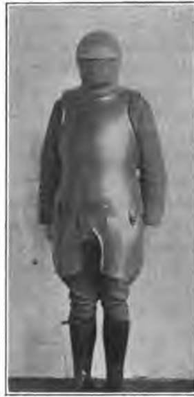
FIG. 202.—The sentinel's armor is combined with the gun proof helmet for protection against sniper's fire.
