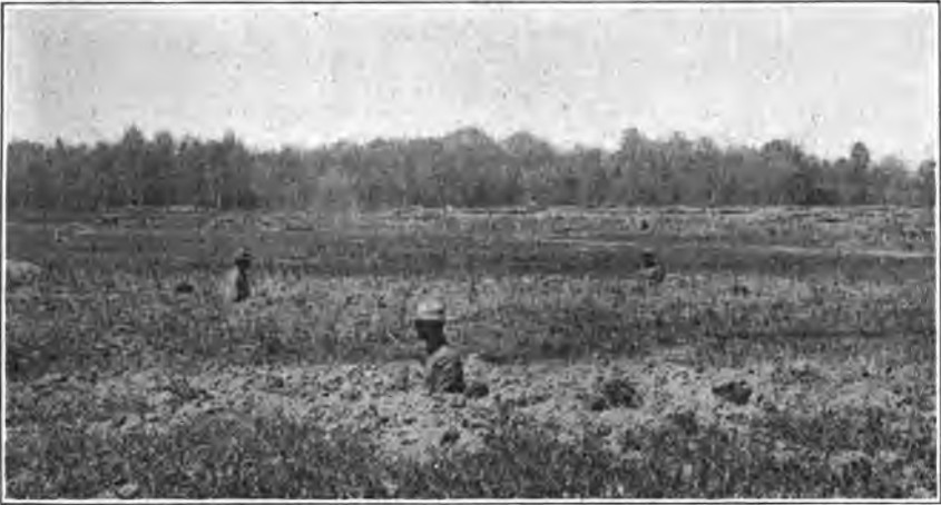
FIG. 101.—Three craters formed by explosion of 6-inch Newton projectiles fired at same angle with delay fuze.
