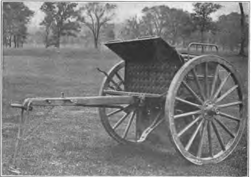
FIG. 11.—3-inch gun caisson, model of 1916, left front view, door open, apron down, fuze setter bracket down.
