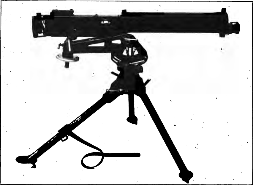
FIG. 136.—Vickers machine gun mounted on a Browning machine gun tripod, model of 1917.
