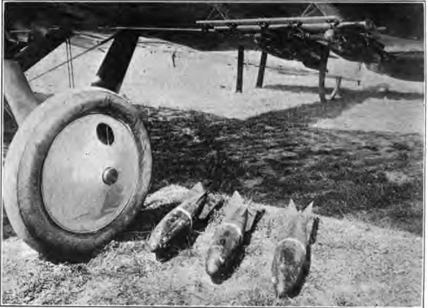
FIG. 125.—Mark III high-explosive bombs and Mark V release mechanism on D. H. 4 airplane.
