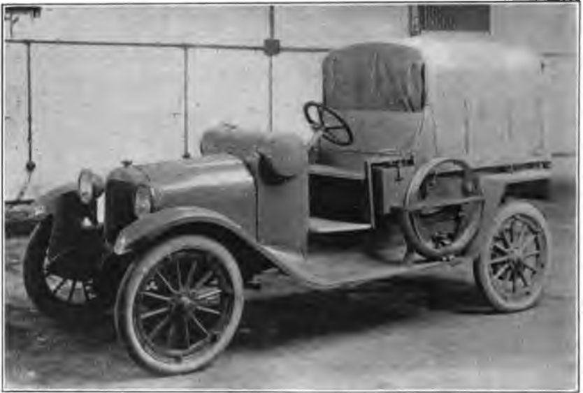
FIG. 100.—Light repair truck on \frac{1}{2} -ton chassis. The type illustrated was later supplanted by an improved model.
