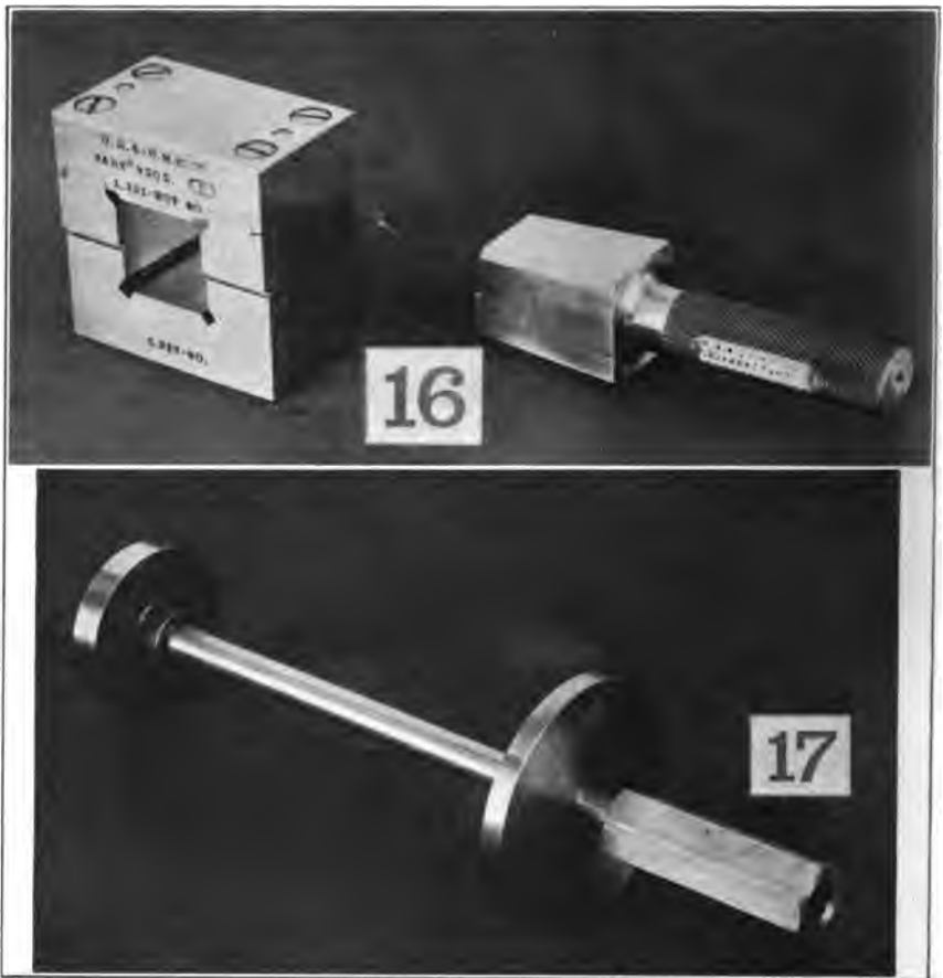
FIG. 220.—Gauges for testing holes or cavities. 16. Square taper gauge and check. 17. Cavity diameter gauge.
