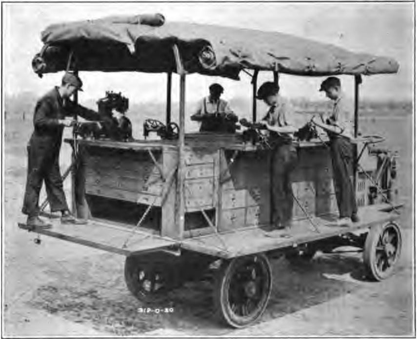
FIG. 170.—Equipment repair truck for making minor repairs of small arms, machine guns, harness, and personal equipment.
