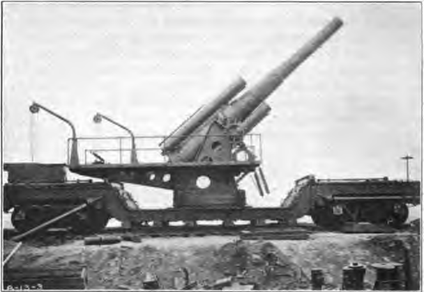
FIG. 31.—8-inch railway mount, model of 1918, showing firing platform formed by crossties laid on H-beams.
