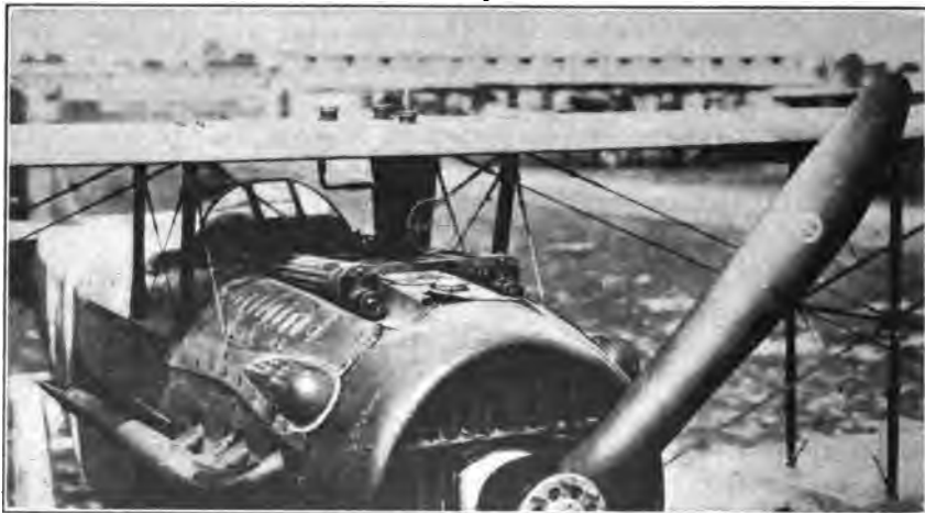
FIG. 111.—Two Vickers guns mounted parallel to motor axis of Spad XIII airplane.
