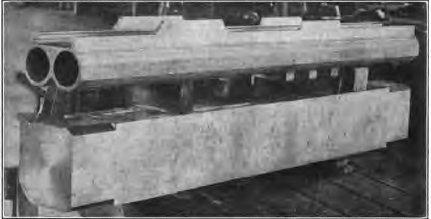
FIG. 4.—Ordnance machining—Spring counterrecoil cylinder for U. S. 75-mm. gun, and steel billet before machining.
