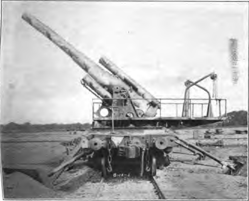
FIG. 32.—8-inch railway mount, model of 1918, arranged for firing at right angles with the track. Note the outriggers and floats.
