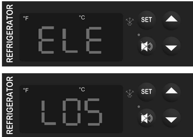
Figure 9. Controller Display Reads "ELE" then "LOS".
