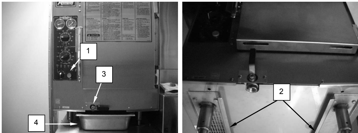
Figure 4. Drain Steam and Hold Oven.
