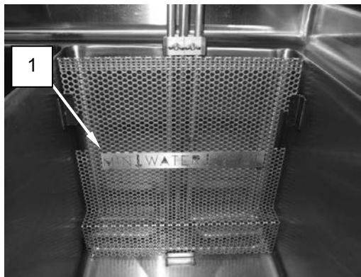
Figure 6. Minimum Water Level for Immersion Heater.
