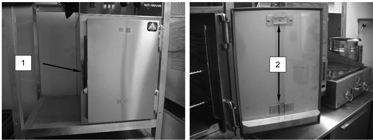
Figure 1. Cook and Hold Oven Vents.
