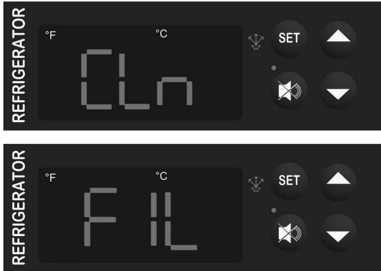
Figure 5. Controller Display Reads "CLn" then "FIL".
