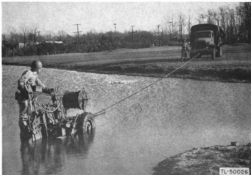
Figure 5. Plow pulled by winch line when crossing stream.
