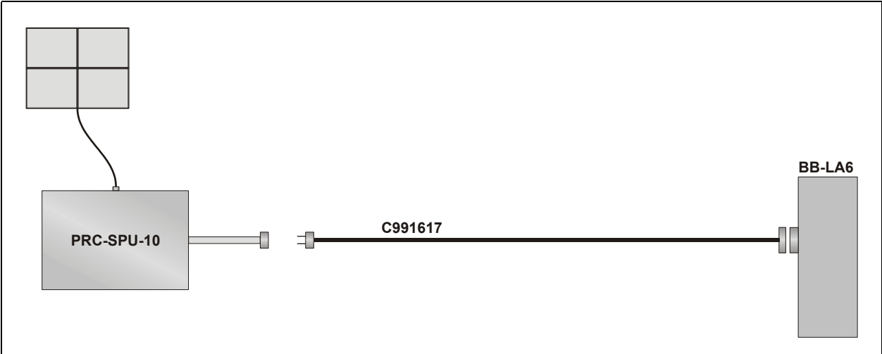
Figure 2-16. PRC-SPU-10 Solar Power Generator with Battery Connected Directly
