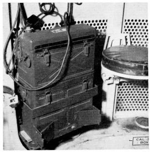
RADIO SET AN/VRC-3-( ) IS MOUNTED IN THE TURRET OF AN M4 MEDIUM TANK.
