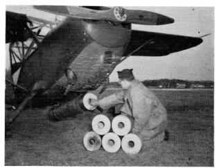
METHOD OF LOADING AIRPLANE COIL CONTAINER.
